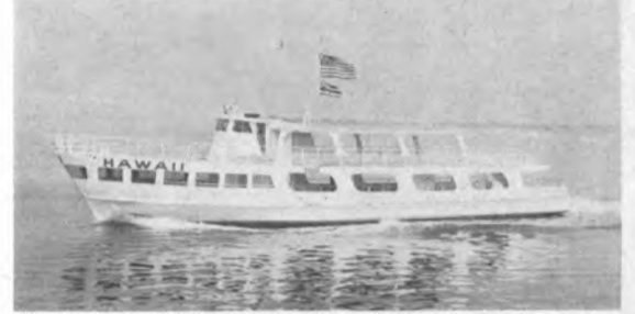
110' PASSENGER FERRY. This 400-passenger Vista View* (wrap-around bow windows. Patent applied for) sight-seeing vessel operates between Waikiki Beach and the Battleship Arizona National Monument at Pearl Harbor.
