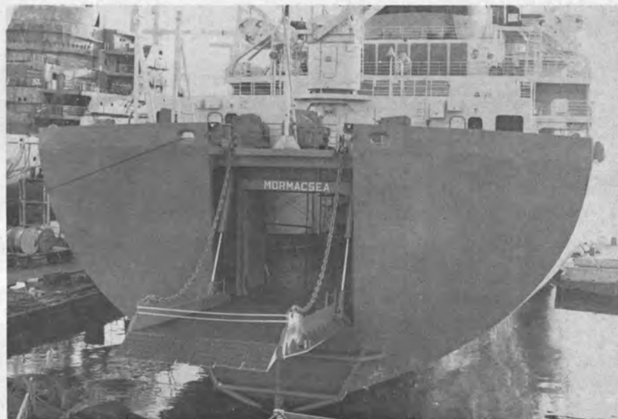
Stern view, with vehicle ramp lowered, shows the passage between the uptakes.
