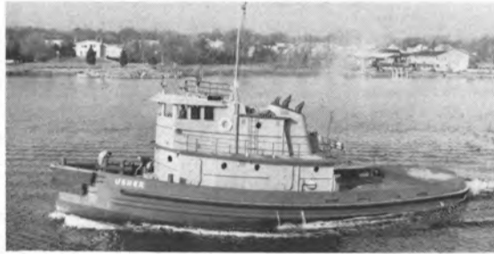
85' HARBOR TUG. Sister ship to the vessel pictured above. Each is powered by twin 765 h.p. diesels and features sleeping quarters and modern galley for a 6-man crew.
