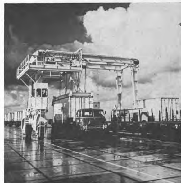
Like the Rotterdam terminal, the Amsterdam container terminal has a direct connection to the international railway system and the vast road network of Europe. Here, containers are transferred between road and rail carriers.
