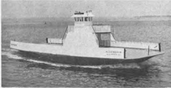
85' DOUBLE END VEHICLE FERRY. Delivered in May, this ferry went into immediate service on Lake Champlain. Fourth in a fleet of Blount double-enders operating on the Lake, she carries 15 automobiles plus passengers on her runs.
