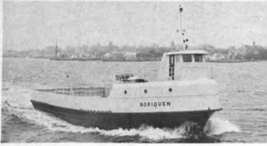
83' PASSENGER-VEHICLE FERRY. This T/L Class vessel is another in the line of Blount Botruc designs. She now operates in regular ferry service carrying 4 trailers and 50 passengers for the Commonwealth of Puerto Rico Ports Authority.
