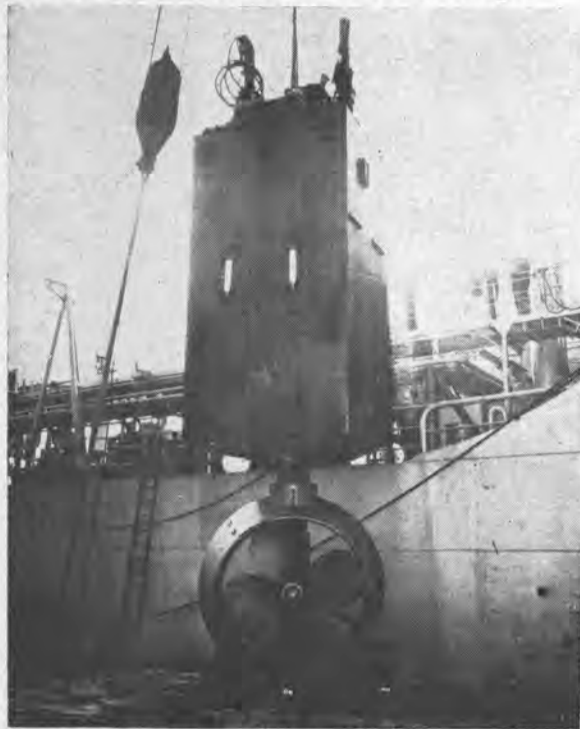
Propulsor pod being lifted aboard Mission Capistrano.
