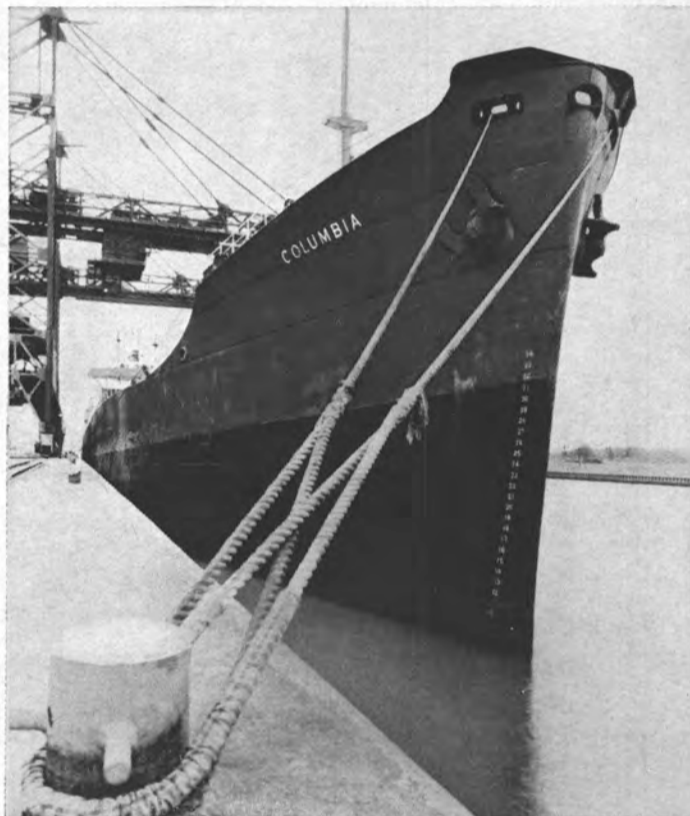
After 3 months' service, there is no fouling, corrosion, or pitting where USS TARSET 305 was applied, below the waterline. Above the line, corrosion, scaling, and pitting of the hull begin to show, despite conventional protective paint.
