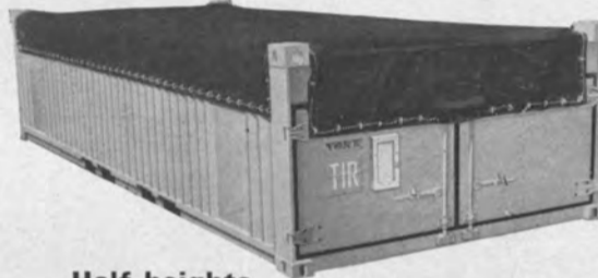
Half-heights 4ft high for high density loads. All-steel ALCHEM-protected. 20, 27, 30 and 40 footers.
