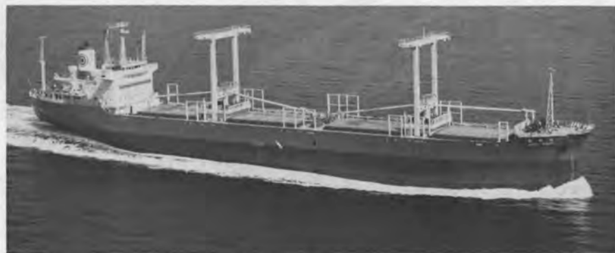
NEW LUMBER CARRIER —Mitsui Shipbuilding & Engineering Co., Ltd., Japan, recently delivered at its Tamano Works the 19,000-dwt lumber carrier, Hiko Maru, to her owners, Sanko Steamship Co., Ltd. The 479-foot ship, which is to ply between Japan and North America, has three sets of 15-ton booms and one 20-ton boom, with strengthened upper deck, hatch coaming and hatch covers. The maximum trial speed of 18.59 knots was developed with the 9,400-bhp Mitsui B&W diesel engine.
