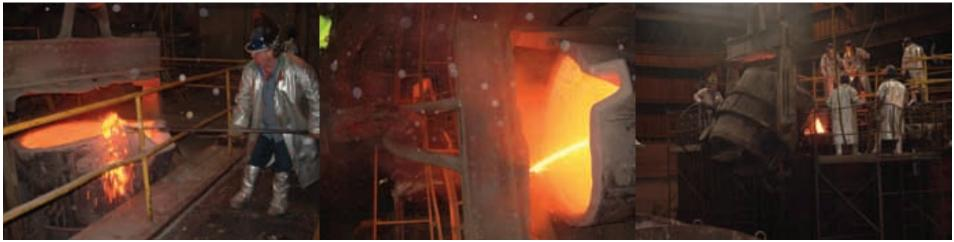
A worker in a fire resistant safety suit draws off a sample of the metal that is taken to an in-house lab for analysis.
