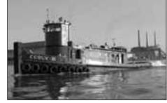
84' Model Bow - Twin Screw Flanking Rudders, Elevating Pilot House Tow Winch - Located in Michigan
