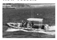
The Ribcraft 6.5 (21 ft.) was introduced this winter. Measuring over 21 ft., this RIB features Ribcraft's signature deep V hull design with full length lifting strakes and integrated internal stringer system as well as Ribcraft's multi chambered Hypalon tubes. Designed with all weather
