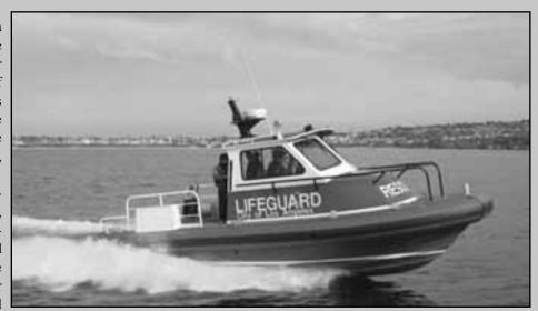
at 315 hp achieving speeds of 29.2 knots. Optional outfitting includes twin dual level controls, air/hydraulic suspension seats, emergency light package, electronics suite, tow line reel and bow storage compartment. To facilitate rescue operations, the boat features a recessed deck area at the transom, a dive door and swim platform.
