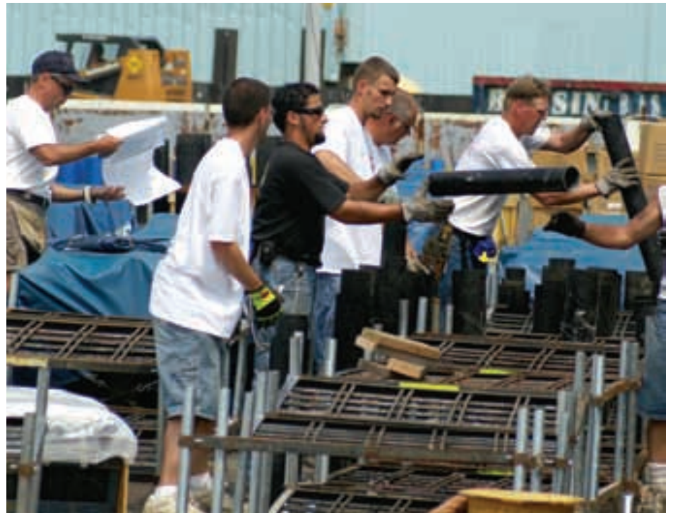
The airborne display begins long before ignition, the crew tossing-along the mortars for exact placement within the patented Gucci frames, there to be wired for ignition from a laptop. The "escape charge" could include up to a pound of black powder. (Photo: Don Sutherland.)
