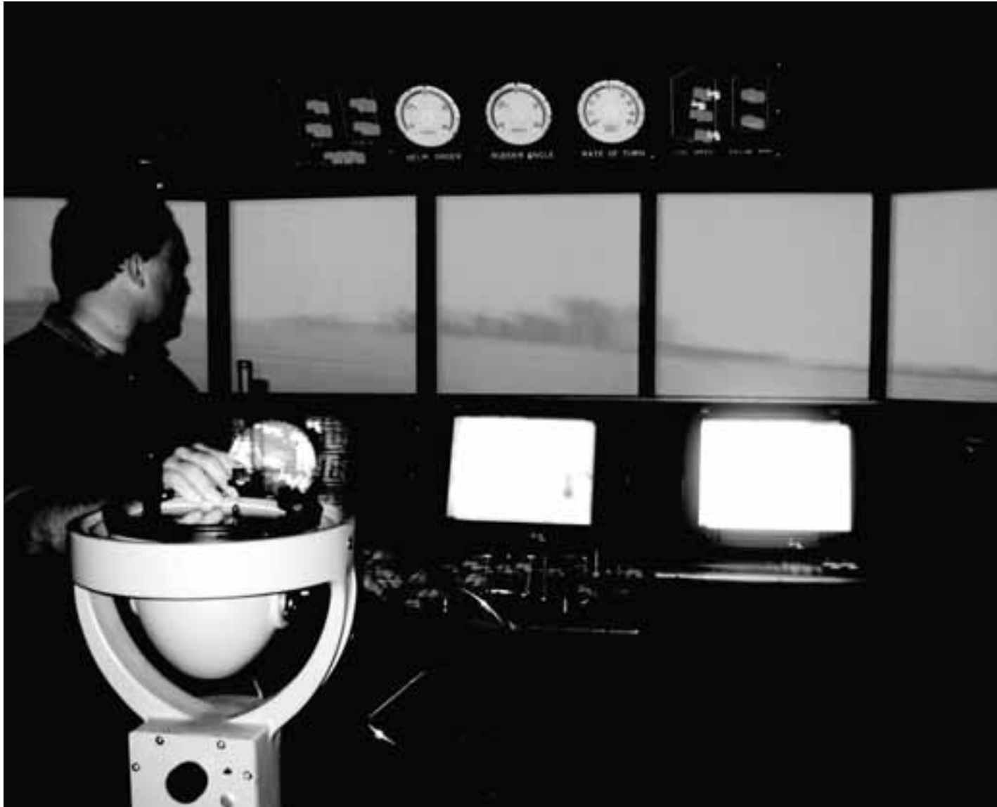
The S.M.A.R.T. Center at MPT employs navigational simulator software from Transas Marine USA and is comprised of three completely interactive full mission bridges one of which boasts a 325-degree curved screen with nine channels of visual projection.
