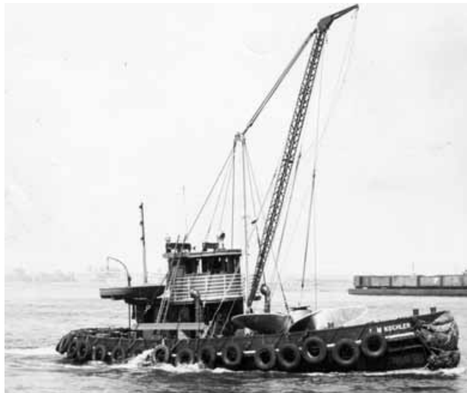
If the Louisiana lugger looks familiar to old-timers, its passing resemblance to the old self-propelled harbor lighter might be an explanation. Here, Kosnac's K.M. Koehler is underway in the mid-1960s, delivering a propeller weighing something around 25 tons. (Photo courtesy K Tugs NY, scan by Don Sutherland.)
