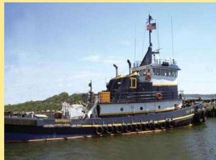
engines for a pair of 1,600 hp Cummins QSK50 engines. The repower involved modifications to the engine foundations and cooling system all of which was carried out at the Lyon Shipyard in Norfolk, Va. The ABS load-lined model bow tug is fitted with an Intercon DD200 towing winch loaded with 2,000 ft of two-inch cable and 305 ft of 1.5-inch wire. It carries tanks for 81,385 gallons of fuel and 5,268 gallons of potable water.
