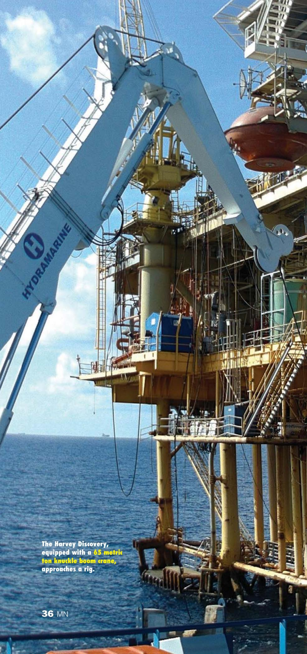
The Harvey Discovery, equipped with a 65 metric ton knuckle boom crane, approaches a rig.
