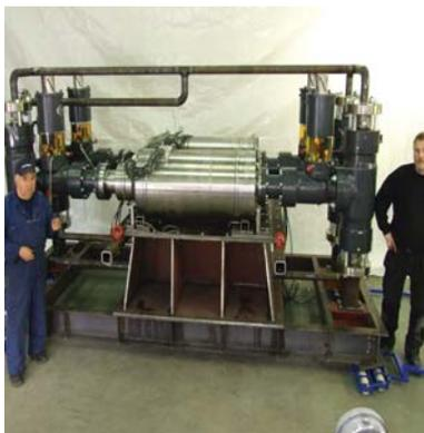
liquid pump is hermetically sealed for zero emissions, has high pressure and capacity, no subsea/topside VSD and is suited for ultra deep water.
