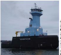
Donjon Marine Co., Inc., along with partner Seacor Holdings Inc. announced the completion of the tugboat, Ken Boothe, Sr. The 10,700 hp tug will work as an articulated tug/barge (ATB) in conjunction with a 34,000 ton capacity self-unloading bulk cargo barge. The tugboat was constructed in the Donjon Shipbuilding and Repair facility over the last 14 months. The still-to-be-named cargo barge is scheduled to be delivered in early Spring of 2012.
