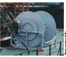
heavy-duty three-inch square tubing frames that are braced at all stress points with two-inch square tubing. The drum of the reel has an open design with a half-inch inner steel plate for reinforcement and a positive pin-lock to lock the reel in place. All boom reels feature #50 chain and sprocket rewind as well as quality-lubricated bearings.
