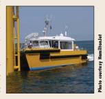
vessel to utilize carbon fiber construction; the 91.8-ft catamaran with twin HamiltonJet HM651 waterjets, currently in build in the UAE at Topaz Shipbuilding.
