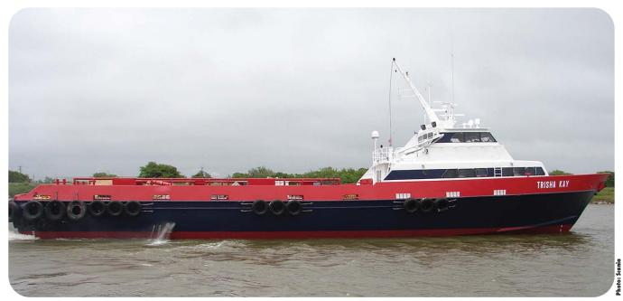
M/V Trisha Kay operating in the Gulf of Mexico is a crew boat with a quadruple installation. The boat is  $130 \times 35$  feet, and is repowered with four Scania DI 16 engines rated at 650 hp each.
