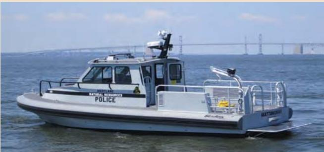
accommodations include electric/pneumatic seating, a full galley, V-berth and a marine head. Mission enhancements consist of a Furuno 1832 Radar, Garmin GPS/MAP 4212 bundle, Hurley infra-red camera, ICOM radio and Wing foam collar. The main propulsion engines are twin Cummins 490 hp, QSC 8.3 inboard engines. For onboard electrical service, a 9.0kW Kohler generator is provided. Fully operational, the boat achieves a maximum speed in excess of 31 knots.
