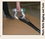
continuous winding of parallel strands of fibres around two end fittings until the right cable strength or required cable stretch has been reached. By maintaining a constant and equal tension (with an accuracy of 0.1%) in all fiber strands during the winding process, an efficiency of more than 80% on the used fibers is reached.
