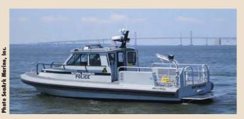
accommodations include electric/pneumatic seating, a full galley, V-berth and a marine head. Mission enhancements consist of a Furuno 1832 Radar, Garmin GPS/MAP 4212 bundle, Hurley infra-red camera, ICOM radio and Wing foam collar. The main propulsion engines are twin Cummins 490 hp, QSC 8.3 inboard engines. For onboard electrical service, a 9.0kW Kohler generator is provided. Fully operational, the boat achieves a maximum speed in excess of 31 knots.
