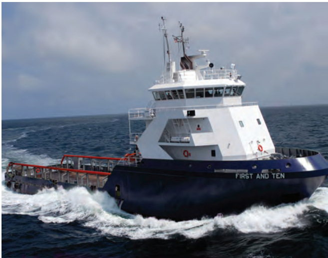
GPA 654 PSV's were the first vessels with the engine room located above the main deck, allowing for 30% more cargo space below deck.
