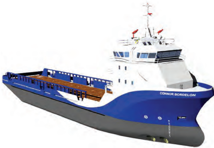
The Stingray design – ABS SOLAS classed, Full Oceans, L&I, ACCU, FIFI 1, DP2, AMS – utilizes special software and a combination of large and small generators to maximize fuel efficiency.
