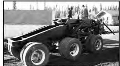
3 axle, 6 ft, 40 ton hydraulic lift fifth wheel dolly
