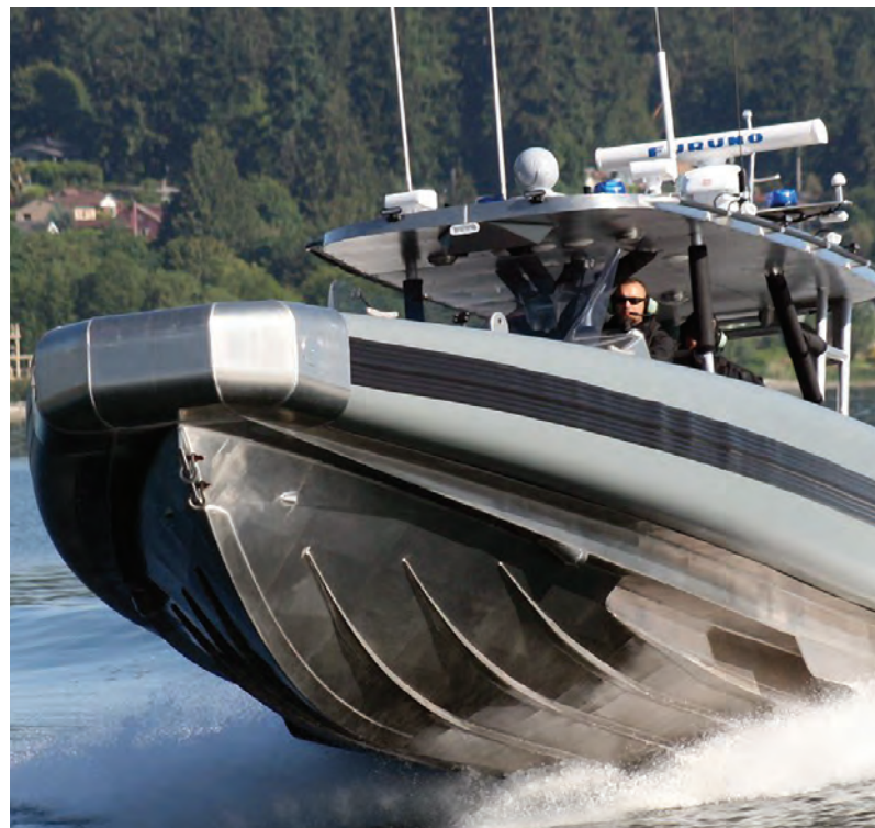
The SAFE Boats 41-foot Coastal Interceptor Vessel (CIV) with advanced design and technology reaches speeds in excess of 54 knots.
