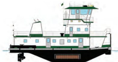
68' harbor tug with Veth VZ-700 Z-drives designed by Sterling Marine, LLC
