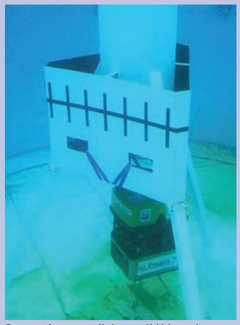
Prototype Autonomous Underwater Vehicle passing through a structure during tank trials, without tether.30 MTR
