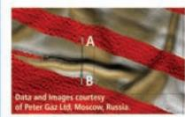
Figure 2 High-resolution Bathymetric data (shown in gold & white), obtained from a towed C3D, is overlaid on multibeam data (shown in red) retrieved from the surface vessel.
