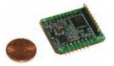
PNI Sensor Corporation announces availability of the MagIC ASIC. When used in conjunction with PNI's SEN-XY magneto-inductive sensors, the MagIC facilitates six times greater magnetic resolution and sample rates than the current PNI solution. The MagIC is a new magneto-inductive drive circuit enabling PNI's SEN-XY to more precisely and rapidly sense magnetic fields while drawing very little power.
