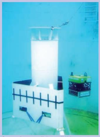
Prototype Autonomous Underwater Vehicle performing a structural inspection during tank trials.
