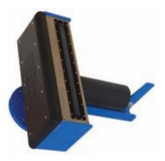
face bottles. The focused  $0.5^{\circ} \times 1^{\circ}$  beam widths, coupled with ultra high 60kHz signal bandwidth, are designed to provide excellent resolution over bottom features and imagery. The Sonic 2024 provides productive swath coverage up to 150° (7.4x WD) with selectable ping rates up to 100 Hz enabling faster survey speeds, reducing survey time and costs.
