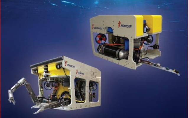
**Sub-Atlantic ROVs** are capable of operating in the harshest environments, offering outstanding reliability and ease of maintenance.
