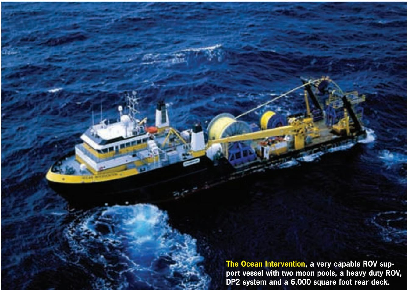
**The Ocean Intervention**, a very capable ROV support vessel with two moon pools, a heavy duty ROV, DP2 system and a 6,000 square foot rear deck.
