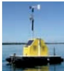
Applications include surface water, drinking water reservoirs, hydropower, and near coastal and ocean research. Multiparameter sondes provide real-time readings for dissolved oxygen, temperature, conductivity, pH, turbidity, and other parameters.
