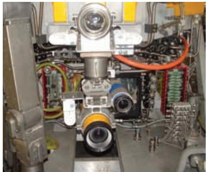
**Lights, camera, action.** This ROV carries several cameras and lights so the operator gets a clear picture of the work being done. Two work arms are at opposite sides of the photo.
