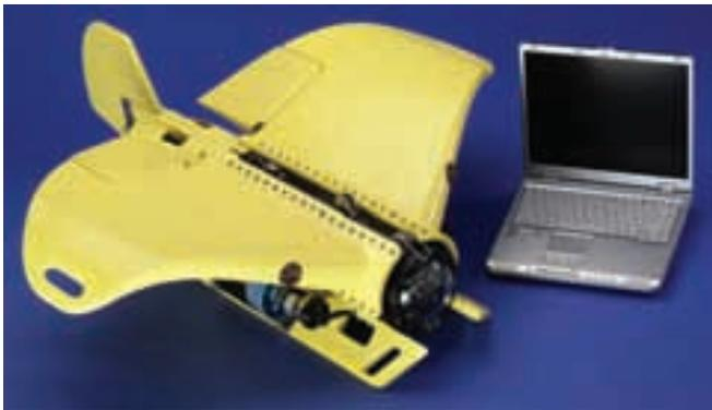
Nova Ray, Inc. offers a line of ROV's for survey, inspection and security applications. All models incorporate the patented arcuate (bow) shaped wing design. The arcuate shaped wings of the Nova Ray are designed to counteract the lifting force of the umbilical, to reduce the effects of boat speed and current on the operational stability. The wings are also designed to increase cable use efficiency and reduce the amount of cable necessary to operate or tow at depth.
