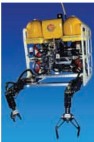
after two years of negotiation by Seaeeye with a subsidiary of the China National Offshore Oil Corporation, (CNOOC). This order is for the 15th Panther to be built by Seaeeye for the oil and gas industry. The unit's stated high maneuverability is achieved with a combination thrust of 220 kg forward and 170 kg lateral through eight vectored brushless DC thrusters
