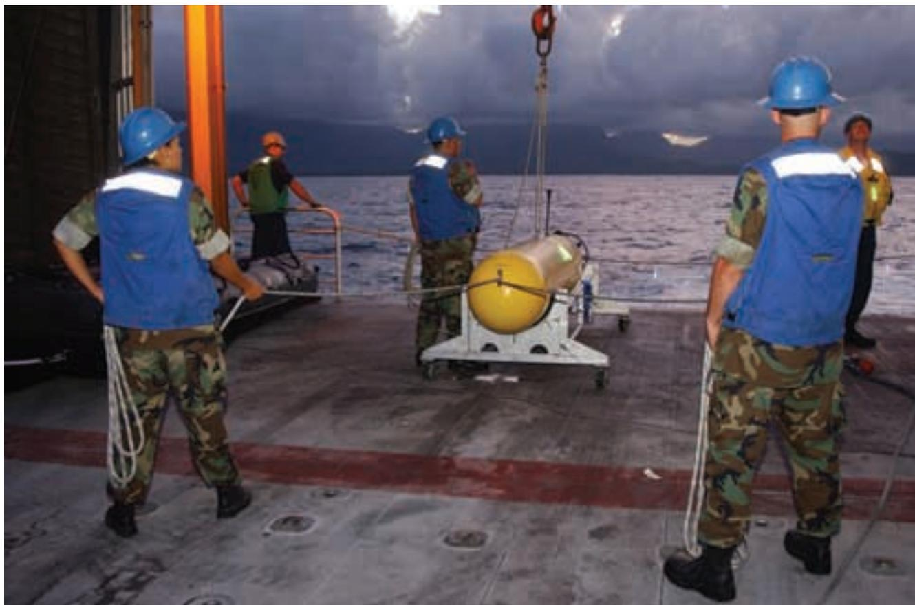
Crewmen assigned to Commander Mine Warfare Command, Unmanned Underwater Vehicle (UUV) Detachment prepare to launch a **Battle-Space Preparation Autonomous Underwater Vehicle**.
