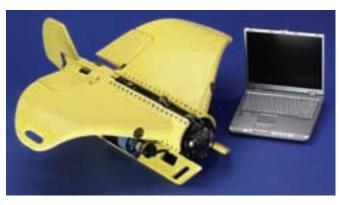
Nova Ray, Inc. offers a line of ROV's for survey, inspection and security applications. All models incorporate the patented arcuate (bow) shaped wing design. The arcuate shaped wings of the Nova Ray are designed to counteract the lifting force of the umbilical, to reduce the effects of boat speed and current on the operational stability. The wings are also designed to increase cable use efficiency and reduce the amount of cable necessary to operate or tow at depth.
