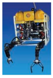
after two years of negotiation by Seaeye with a subsidiary of the China National Offshore Oil Corporation, (CNOOC). This order is for the 15th Panther to be built by Seaeye for the oil and gas industry. The unit's stated high maneuverability is achieved with a combination thrust of 220 kg forward and 170 kg lateral through eight vectored brushless DC thrusters
