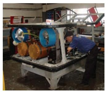
An ROV under construction at the Oceaneering facility. Two ROVs can be built simultaneously in this area.
