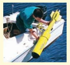
hunters, marine archeologists, commercial diving companies, law enforcement agencies, and military units. The proton mag is designed to be a rugged, reliable instrument that is very easy to operate. In addition to finding shipwrecks, mags are often employed to locate pipelines, anchors, sunken automobiles, weapons, and unexploded ordnance.
