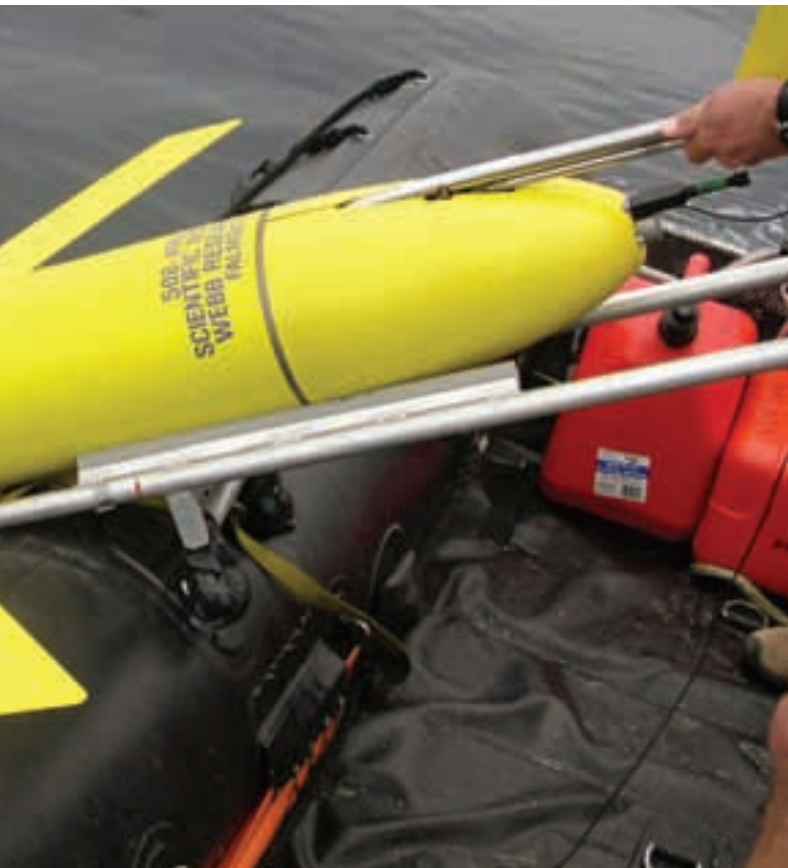
The Mid-sized Autonomous Research Vehicle (MARV), developed by Naval Undersea Warfare Center (NUWC) Division Newport, demonstrated underwater color video survey capabilities, high-accuracy inertial navigation, and interoperability with Solar AUVs (SAUVs) using acoustic communications.
