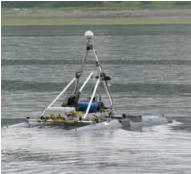
The Hydrographic Unmanned Survey Craft (HUSCy) USV, operated by the Naval Oceanographic Office, demonstrated capabilities for tactical data collection for shallow water hydrography / oceanography and also remote launch of a small Ranger RN-2 UUV, a demonstration conceived during AUV Fest 2005 by the two vehicle teams in the collaborative environment fostered by the National UUV T&E Center concept.
