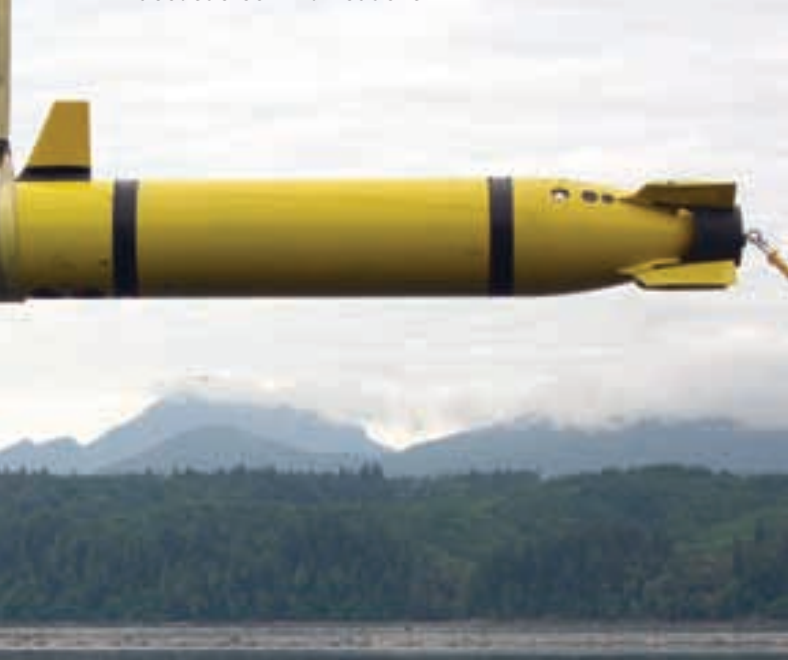
The Mid-sized Autonomous Research Vehicle (MARV), developed by Naval Undersea Warfare Center (NUWC) Division Newport, demonstrated underwater color video survey capabilities, high-accuracy inertial navigation, and interoperability with Solar AUVs (SAUVs) using acoustic communications.
