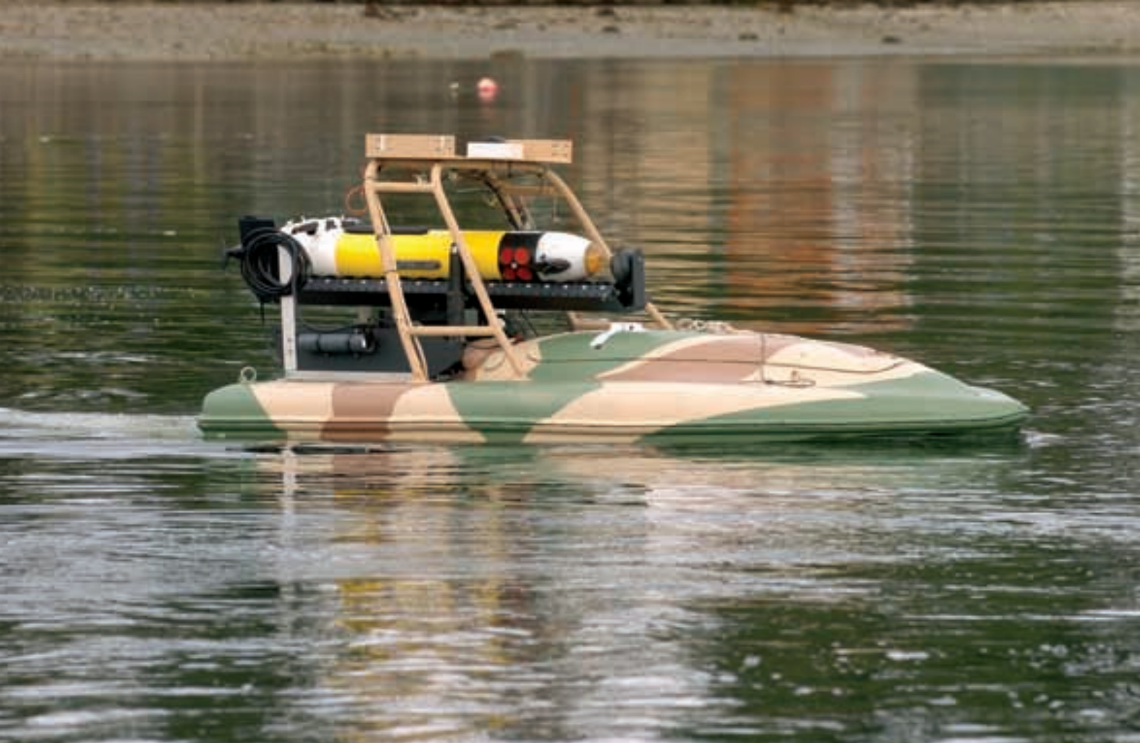
The Remote Delivery of Unmanned System Technology (RDUST) project from Naval Surface Warfare Center (NSWC) Panama City demonstrated a capability to launch a REMUS UUV from an Autonomous Search and Hydrographic Vehicle (ASH) USV, as could be used to rapidly insert a slower-speed UUV into a distant mission area.
