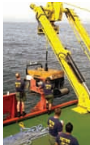
Official U.S. Navy file photo of the "Super Scorpio" remote operated vehicle (ROV) to a safe recovery aboard the special mission charter ship M/V Kellie Chouest. U.S. Navy photo by Photographer's Mate 1st Class Daniel N. Woods
