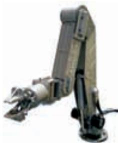
arate enclosure to the manipulator forearm, eliminating the subsea slave controller, slave cable, and 79-pin wiring harness. The new design also reduces Titan system weight by approximately 18 kg (40 lb) in air and 9 kg (20 lb) in water. The standard depth rating has increased to 4,000 m, and a 7,000-m model is also available.
