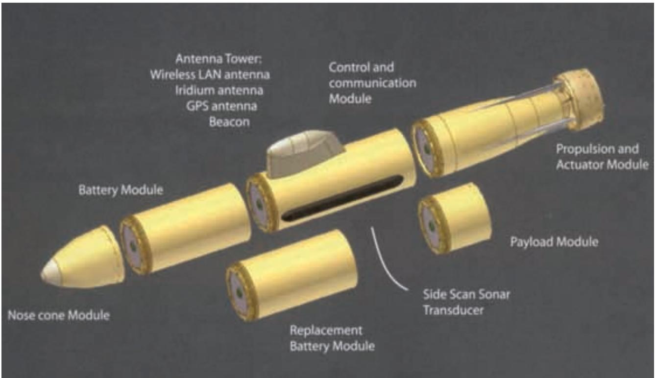
fitted together by the user, using Gavia's patented QuickLock system. "Other companies offer modular designs, but ours is the only one that is put together by the user," said Steingrímsson. "With all others, the reconfiguration must be done at the factory."
