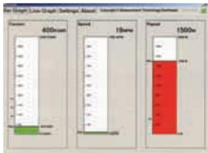
a serial interface to a central PC with optional touch-screen display. The program has the ability to log and summarize data for each winch and cast, replay the time history plot for any parameter from past casts on a second screen, calibrate winch tension and count sensors directly from the central computer, and allow operators to customize the display to their specific requirements.
