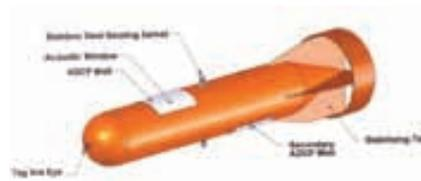
The Flotation Technologies StableMoor is designed to reduce drag and increase mooring stability in extreme flow regimes. With a theoretical drag coefficient of 0.3, StableMoor is a solid syntactic foam, torpedo-shaped buoy featuring a new stainless steel mooring swivel to provide smooth transitions to changes in current direction.
