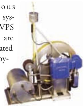
down to 300 m, or may be installed on moored subsurface buoyancy platforms in deep water applications. They are fully automated and feature stainless steel construction, underwater mateable connectors, pressure compensated (oil-filled) components, premium slip ring assemblies, regulated power systems, and serial interface for diagnostic, control, and command functions.
