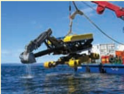
Nexans has developed a terrain dredger/sub-sea intervention system called the Spider. The Spider combines powered tracks with an articulated walking leg system, enabling it to function in uneven sub-sea terrain with up to 35 degrees slope. It is built to work in water depths of approximately 1,000 m. The Spider's movements are controlled by operators located aboard a support vessel, it is launched via a specialized Launch & Recovery System (LARS). Power and signals between the vessel and Spider
