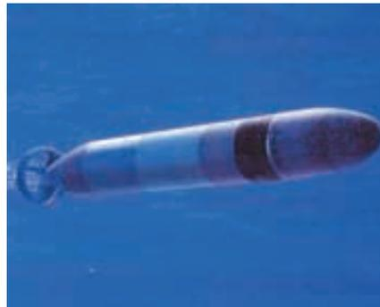
fidelity to be used either on range or in the open ocean. It is a small submarine-like target equipped with acoustic and non-acoustic signatures and can be deployed from an underway submarine to enhance fleet readiness in anti-submarine warfare.
