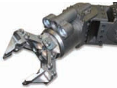
Schilling Robotics' new integrated wrist camera for TITAN manipulators features a titanium camera housing for protection and internal cabling that is designed to eliminate cable snags and abrasions. The high-resolution color camera, which includes LED lights with two illumination levels, can be ordered in either NTSC or PAL format. The depth rating is 4000 m.
