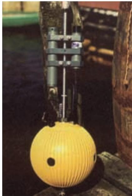
data is converted from the time domain to the frequency domain and analyzed using Fast Fourier Transform (FFT) techniques. The directional wave information is available as output from InterOcean's Wave for Windows analysis software or may be output directly from the new generation S4ADW-I which processes this data internally for immediate availability to the user without the need for external software.
