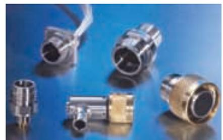
and alloys are available upon request. Bulkhead connectors are available in threaded or flanged versions with a removable glass reinforced epoxy insert, and straight and right over-molds are available for cable connector plugs. The connectors have up to a 10,000 psi pressure rating in mated condition; the bulkhead connector design open face is rated to 5,000 psi.
