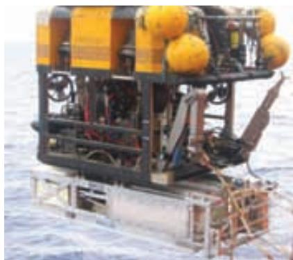
Commissioning System (SPCS) known as Denizen. Designed for ultra deepwater applications, Denizen is operated in conjunction with a work class Remotely Operated Vehicle and currently has the ability to work in water depths to 10,000 ft. and achieve pressures up to 20,000 psig.
