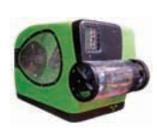
underwater surveys of tight interior spaces. The SpiderBot ROV is suited for work considered too dangerous or inaccessible for divers, larger ROVs, or manned submersibles. The system provides high-resolution imaging, close-in inspec-
