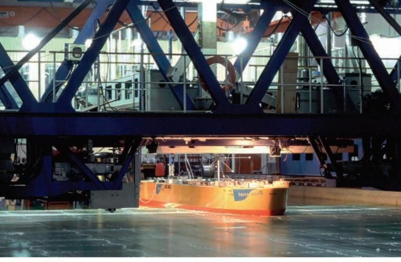
The Ice Tank in St. John's is the world's longest refrigerated indoor pool. NRC researchers use it to study the design of vessels and structures that operate in ice-covered waters.
