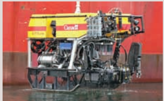
The ROPOS Remotely Operated Vehicle is equipped with the IXSEA Global Acoustic Positioning System (GAPS).
