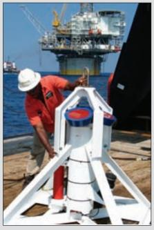
BroadBand processing for significantly improved data quality, power efficiency and error detection; a patented two (2) dimensional phased array transducer design for significantly reduced size, weight, and deployment complexity; and a unique 4-beam configuration to ensure data quality and reliability.
