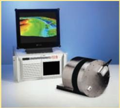
A bathymetric sonar operating at 240kHz, the SeaBat 7101 measures discrete depths over a wide, 150° swath to a maximum range of 500m. A true, time-delay beamformer uses a combination of amplitude and phase detect for maximum performance across the entire swath. Roll stabilization maximizes efficiency during survey operations. Dense sounding coverage is achieved with a combination of
