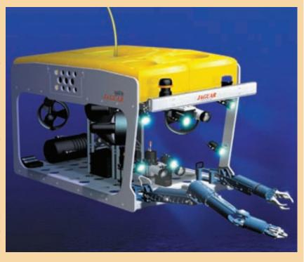
There is also a new dual redundant high-frequency/high voltage power distribution system, allowing the ROV to continue to operate on reduced power if one of the dual power systems fails. It also reduces the diameter and weight of the umbilical, and significantly cuts the size and weight of the onboard transformer.
