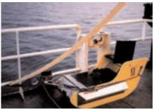
non-conducting cable. Its undulation instructions are preloaded into the built-in controller, which is powered by the vehicle's impellor driven alternator, which allow deployment from ordinary winches and capstans. Real-time flight control and data acquisition can be obtained via conducting cable.
