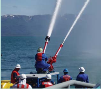
T&T Bisso team delivering 6000 gpm during offshore firefighting deployment exercise.
