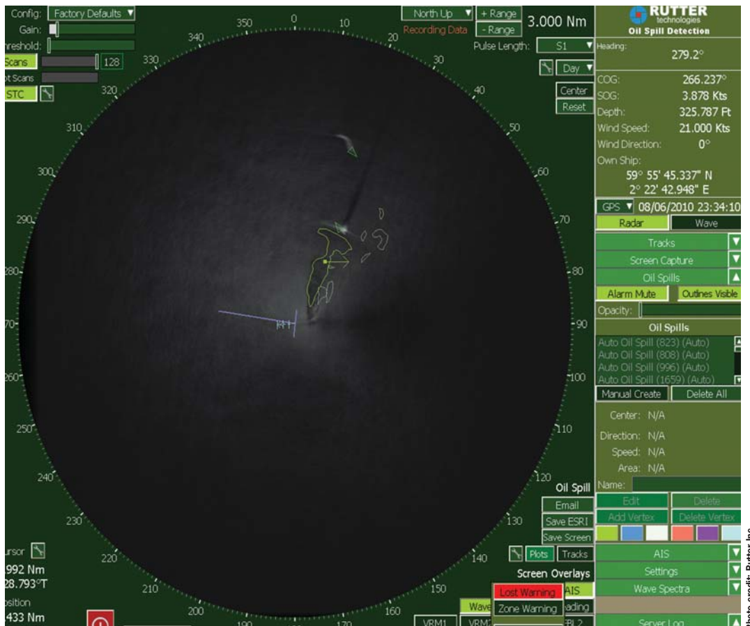
Rutter’s Sigma S6 Oil Spill Detection system: Outlined shapes show oil spills actively being tracked. Arrow pointing east from green outlined section shows drift direction. Triangles show the location of other vessels.
