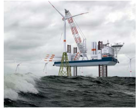
Wärtsilä and Aker Solutions jointly developed a High Performance Turbine Installation Vessel. This HPTIV can operate in year around weather conditions with an operational water depth range of 4.5-50m.
