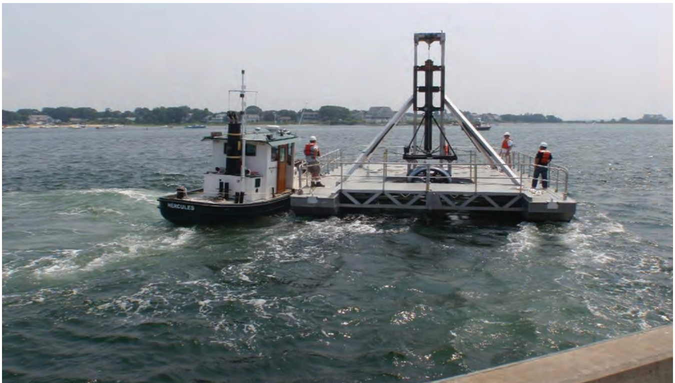
Free Flow Power's turbine being towed to the Massachusetts Maritime Academy's partial scale test site aboard the barge donated by Verdant Power, New York, NY.
