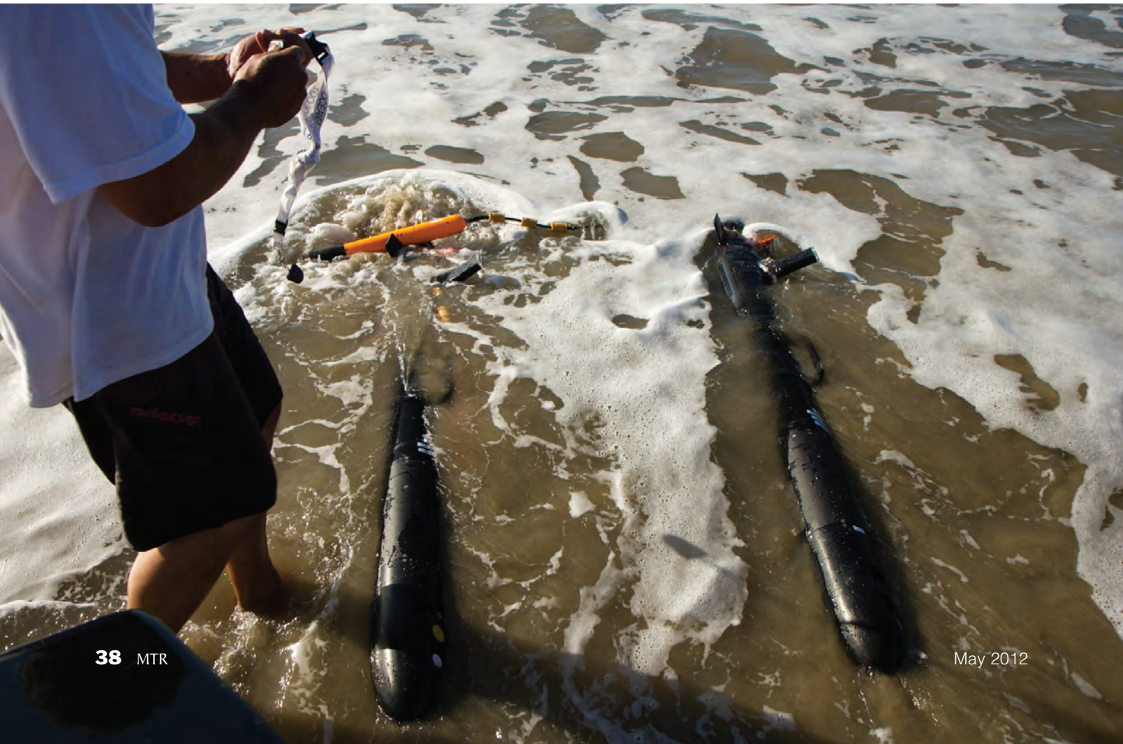
AUVs swim through the surf zone for beach recovery.
