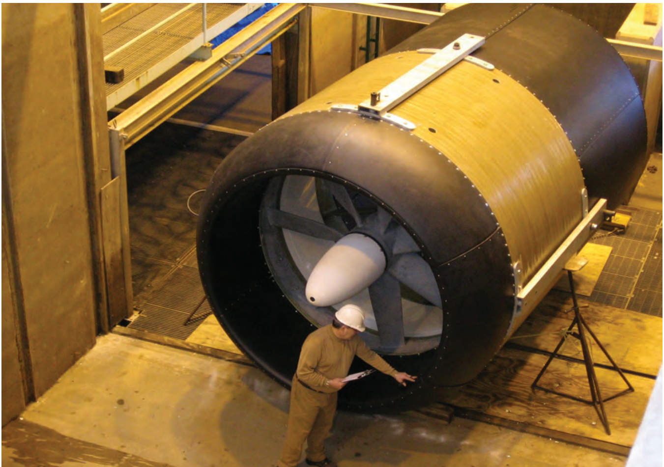
Free Flow Power's turbine being tested at USGS Conte Fish Center, Turner Falls, MA
