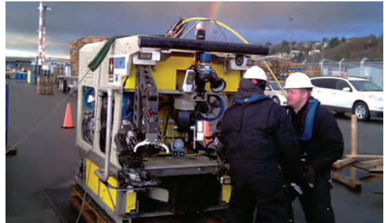
Engineers prepare the ROUMRS ROV, equipped with a WSM 6 transponder, ready for deployment
