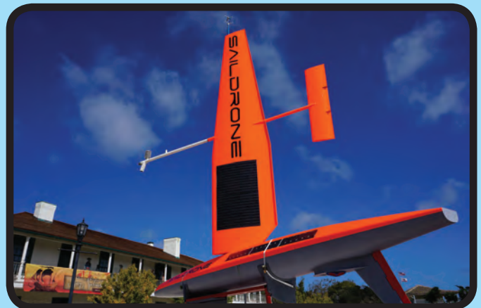
The wind and solar powered SAILDRONE autonomous surface vehicles are built in Alameda, CA.
