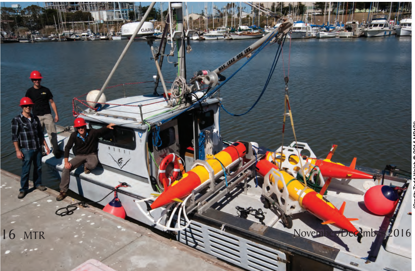
MBARI engineers Ben Yair Raanan, Brian Kieft, and Brett Hobson prepare to deploy three long-range autonomous underwater vehicles from the Research Vessel Paragon in Monterey Bay.
