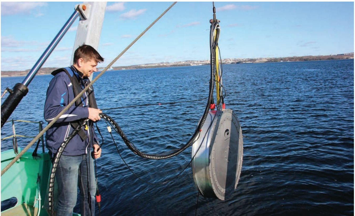
Deployment of a C-BASS VLF sound projector: a recent product launch from GeoSpectrum Technologies that fulfils a range of operational roles for the marine sector.
