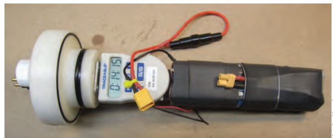
Figure 8 A 100-hour scientific countdown timer is adapted for a time release. The 1.5vdc signal that powers the beeper is used as the gate input to a SCR. The 9.6vdc NiMH battery pack supplies power to a burnwire. Similar timers in 7075 aluminum housings have been used to the bottom of the Kermadec and Tonga Trenches.
