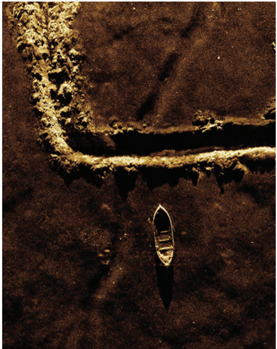
Image of 7-meter Dory and Anchor Scar taken from HII REMUS with MINSAS 60.
