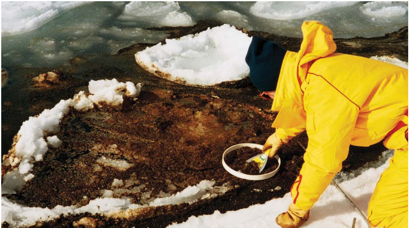
Sampling oil on the surface of pancake ice during a 1986 field experiment off the Canadian East Coast.
