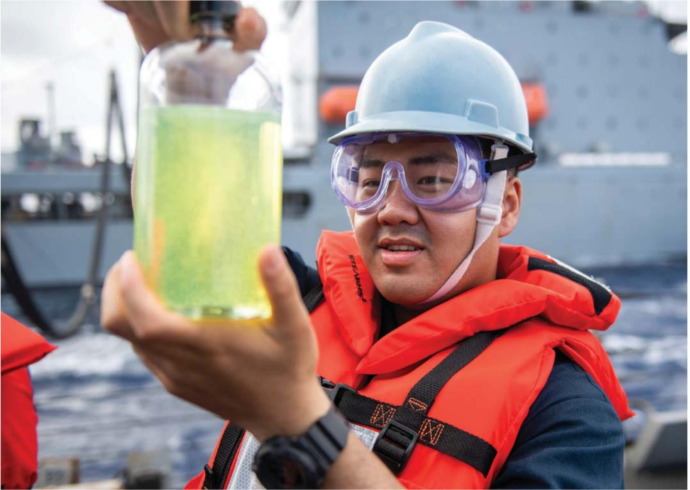
Gas Turbine System Technician (Mechanical) 3rd Class Raymond Htut inspects a fuel sample for color and clarity aboard the Arleigh Burke-class guided-missile destroyer USS Curtis Wilbur (DDG 54) during a replenishment-at-sea with the fleet replenishment oiler USNS John Ericsson (T-AO 194)
