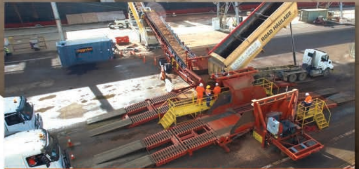
ONE TO THREE LANE PORTABLE TRUCK UNLOADERS
