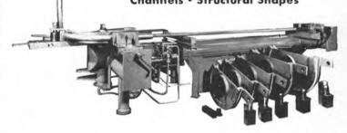
They are easy to operate. Only two levers to use one to do the bending and reversing—the other operates the mandrel—in or out! The mandrel unit is optional.
