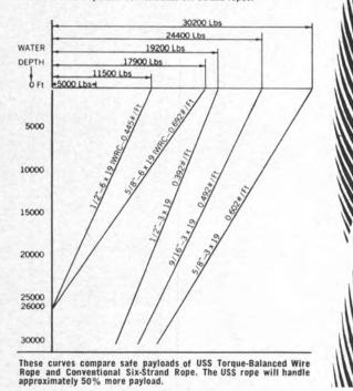
Rotation, kinking, unwinding, breakage and corrosion are the major problems encountered in virtually every oceanographic hauling, hoisting, rigging, mooring or sounding application. USS TIGER BRAND Torque-Balanced, Three-Strand Wire Rope is the answer to these problems of modern deep ocean exploration.
