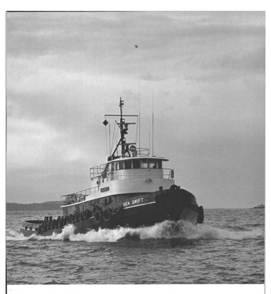
The twin-screw Red-Stack tug, Sea Swift is powered by two General Motors 16-645E5 Diesel engines which are controlled from the pilot house by GM pneumatic control equipment. In calmer seas, she can cruise at 15 knots under tow.
