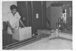
Technician at Nippon Kokan monitors operation of computer-controlled equipment automatically preparing hull form line drawings for ship designs and cost estimates.
