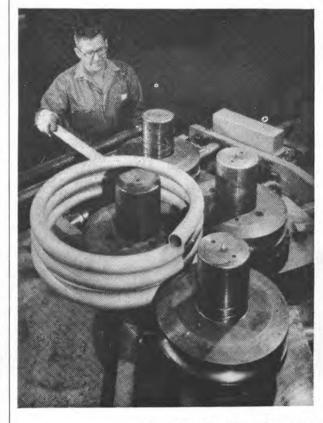
This Wallace 464 Series Rolling Machine is making tight coils in ONE pass through the machine.
