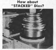
Want to reduce set-up time? Use — ''STACKED'' dies. Here's a typical combination for bending  $-\frac{3}{8}'' - \frac{1}{2}''$  or  $\frac{3}{4}''$ pipe without any changes. Other combinations available.
