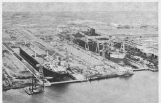
The capacity of our Sakai Shipyard has been vastly increased with the completion last October of a new 400,000 DWT dock. It can easily accommodate the largest ships afloat today. The dock measures 380 meters in length, 62 meters in width and 12.5 meters in depth and is equipped with the latest facilities for ship repair.
