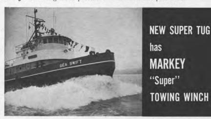
This is how the new super-tug "Sea Swift" entered service — with a king-sized bone in her teeth. As the West Coast's most powerful tug, she needed a winch capable of handling the largest tows. Markey Machinery supplied it. This 2-drum Markey (Model TDSD-36) is diesel-powered, with hydraulic back-up drive. Port drum carries 2,200 feet of  $2\frac{1}{2}$ " wire; starboard drum, 2,600 feet of  $2\frac{1}{8}$ " wire. Markey keeps pace with the trend to larger, faster tugs!
