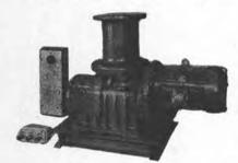
MOTOR: 10 HP-totally enclosed-fan cooledcontinuous duty — horizontal flange mounted — special shaft & oil seal fitted—440/3/60—1760 RPM. CONTROL: Marine type water-tight pushbutton—forward/reverse/stop—watertight starter
