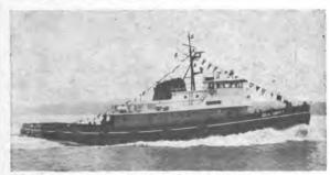
Sea Swift, and sistership Sea Flyer, at 7,000 hp each, are the most powerful vessels of this type on the Pacific Coast. These new oceangoing tugs were constructed at McDermott Shipyard, Morgan City, La., and are now part of the Red Stack fleet operated by Puget Sound Tug & Barge Company of Seattle, Wash.
