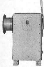
Designed for use with Bathythermograph—Submarine Signal Co.—type E/2/S—without cobles—single speed 300 lb. pull @ 360 FPM—single drum 9" X 63/4"—with 147/8" flanges—clutch controlled with pawl & ratchet. Designed for use with 1200 ft. of 1/8" stainless cable. Motor: 3 HP—440/3/60—1700 RPM—intermittent. 5 Availabe—Navy surplus—show little use.
