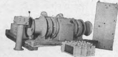
Made by Ideal Electric Co.—with spares. Double wildcat—1-5/16"—15 HP—115 volts DC—1750 RPM—all controls—two outboard gypsies. Wildcats 36" between centers—6000 lb line pull @ 50 FPM. DIMENSIONS: O.A. width over gypsies—84"; OA length 81". Will sell windlass without power if desired.
