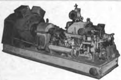
FARREL-BIRMINGHAM, as orig. used on two 1375 HP electric motors, in submarine, 2 pinions, single output gear, Pinion RPM 1302, Gear RPM 280; ratio 4.65:1.
