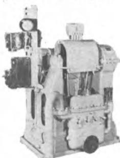
**MOTOR DRIVEN RECIPROCATING BILGE PUMP WITH AIR DOME**
