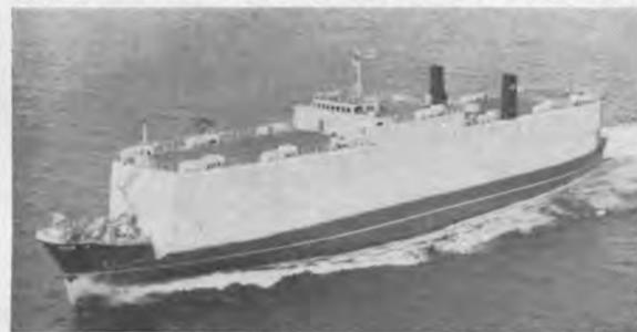
Aoi Maru can carry 737 Toyopet cars. The 380-foot 4-inch vessel has a beam of 53 feet 2 inches, molded draft of 16 feet 5 inches. It is equipped for stern loading.
