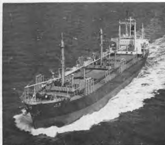
**LOG/BULK CARRIER HALO**, which was built at Hitachi Zosen's Innoshima shipyard, has been delivered to her owner, Liberian Halo Transports, Inc. The 564-foot 4-inch vessel is built to the shipyard's economical standard design with sufficient stability for deck loading of logs. The 23,547-dwt ship is propelled by a Hitachi B&W 762-VT2BF-140 diesel engine developing 8,400 bhp and giving the ship a service speed of 14.5 knots.
