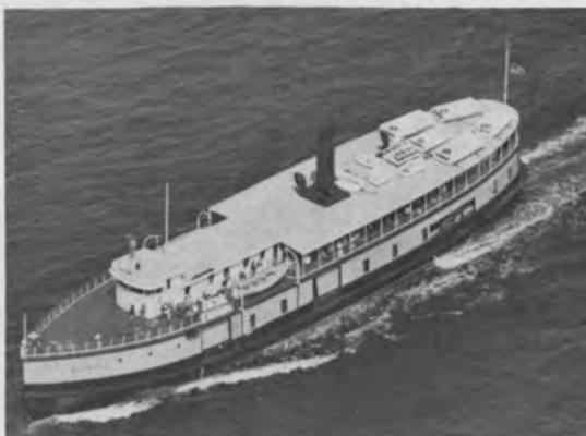
Official Number 223,190. Built 1923 at Staten Island Shipbuilding Company, Port Richmond, N.Y. Steel hull—one deck. Machinery: 3 cyl.T.E.-IHP—1400
