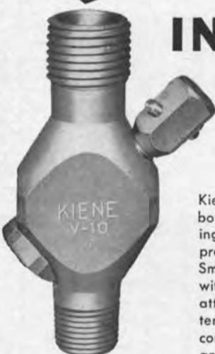
Kiene valves have effective gas seal both open and closed without packing or glands. Operates against pressure — will never blow open. Small and rugged — 4 1/4" in length with only 3 1/4" circle of space for attachments. Kiene valves give better service under the most severe conditions. Standard indicator plug and wing nut connection.
