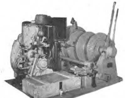
Small general purpose winches, mfg by Jaeger. Rated 2500 lbs @ 75 FPM. Driven by air-cooled Enfield single Cylinder diesel engine. Deutchable free spooling drum has center flange which can be removed if required. Excellent for small vessel use and general purpose service on all vessels. Has spare parts box. Weight about 1500 lbs.
