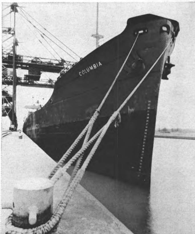
After 3 months' service, there is no fouling, corrosion, or pitting where USS TARSET 305 was applied, below the waterline. Above the line, corrosion, scaling, and pitting of the hull begin to show, despite conventional protective paint.
