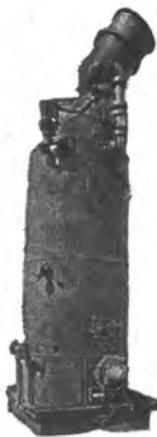
100 HP @ 100 PSI. Water heating surface 747 sq. ft.—total heating surface 1144 sq. ft. A.S.M.E. Built by International Boiler Works—East Stroudsburg, Pa. Height to top of cylinder 12' 0"—diameter 66"—4" main steam line—2 1/2" safety valves—practically new—very little if any use. Oil burning. Boiler stamped Mass.—Standard—100#—5290—National Board No. 6395.
