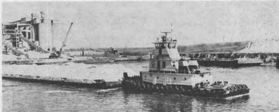
The entire power requirements for the Robin Rose were designed and supplied by Stewart Stevenson. The boat can push three 200-foot light barges at 10½ miles per hour and 8 miles per hour loaded.
