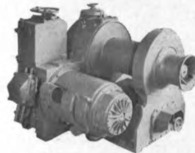
10 A.E.G. Unit-Type Winches—with all controls attached to winch. In very good condition—removed from vessel run for only 1 year. 3-Ton capacity—25 H.P.—230 volts D.C.—Priced to sell!!
