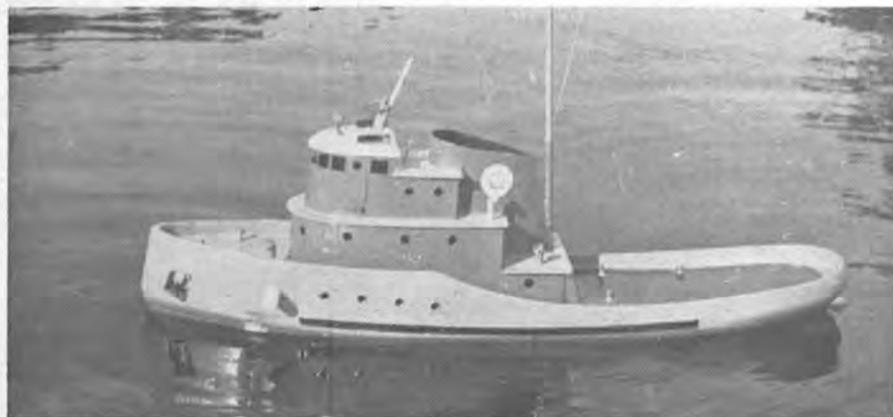
Model of tug with hydraulically operated connection extended just forward of house.
