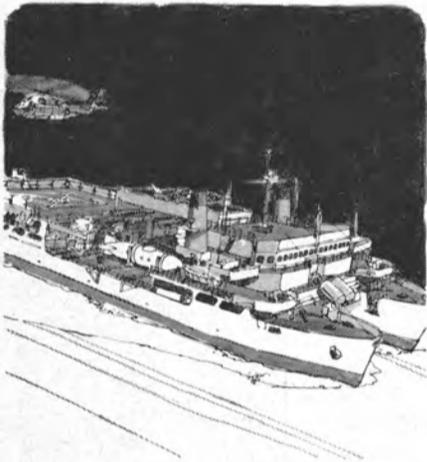
The Navy's first new sub-rescue/deep ocean salvage ships—250' long catamarans—will have an intricate recovery system designed and built by Western Gear.
