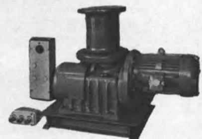
MOTOR: 10 HP—totally enclosed—fan cooled—continuous duty—horizontal flange mounted—special shaft & oil seal fitted—440/3/60—1760 RPM. CONTROL: Marine type water-tight push-button—forward/reverse/stop—watertight starter box—rated for 40 starts per hour—triple pole contactor with silver contacts, thermal overload relay and trip adjustment. DIMENSIONS: Barrel 10" diameter—Flange 10" diameter—approx. 26" wide and 36" long.
