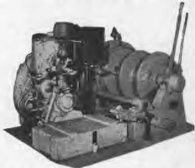
Small general purpose winches, mfg by Jaeger. Rated 2500 lbs @ 75 FPM. Driven by air-cooled Enfield single Cylinder diesel engine. Declutchable free spooling drum has center flange which can be removed if required. Excellent for small vessel use and general purpose service on all vessels. Has spare parts box. Weight about 1500 lbs.
