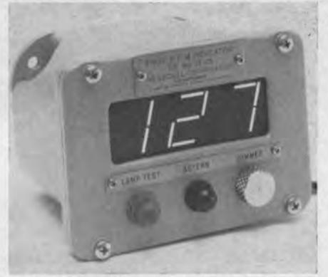
Propeller rpm indicator by Henschel.
