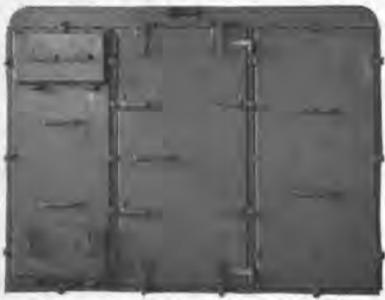
(7) 50 HP—230 volts DC—right hand—mfg by Allis-Chalmers. Resistors, control and brake. Dwg EK9231—U.S.M.C.—820-2—1404 ALT.
