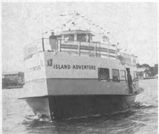
**65' PASSENGER FERRY.** Another successful 2-deck model. This 350-passenger vessel plies Casco Bay, Maine in regular service with 5 sister ferries of Blount design.
