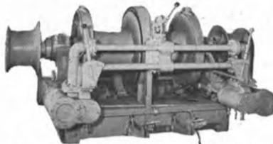
Drum 8500 lbs @ not less than 120 FPM; 13,000 lbs at no specified speed. Gypsy head 22,500 lbs. static pull. Foot brake to hold 17,000 lb. pull. Steam cylinders with standard 250 PSI.
