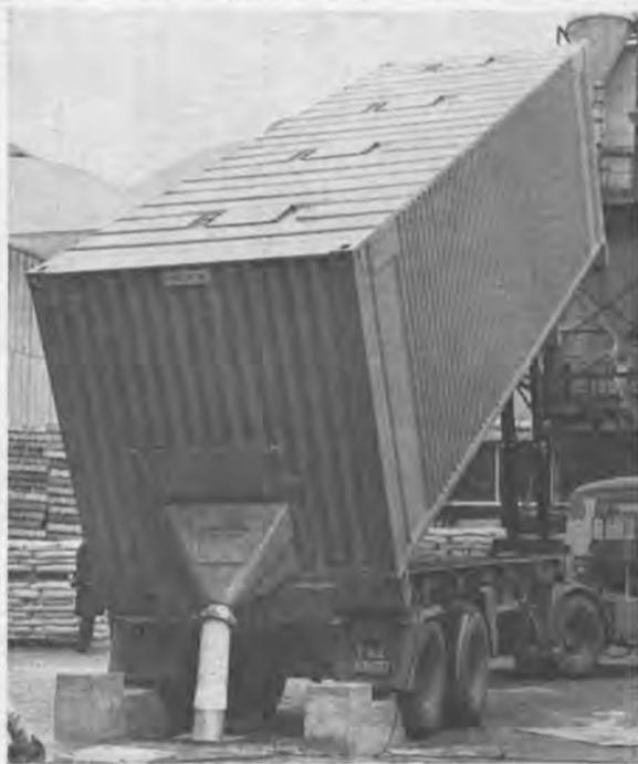
International Ferry Freight Ltd. (I.F.F.) of England has developed in conjunction with I.C.I. plastics division a system for carrying granular chemicals in bulk in standard ISO box containers, which are back-loaded with general freight, thereby eliminating the costly return of empty containers. The containers and tipping skeletal trailers used in the system are being manufactured and marketed by York Trailer Company Ltd., Corby, Northants.
