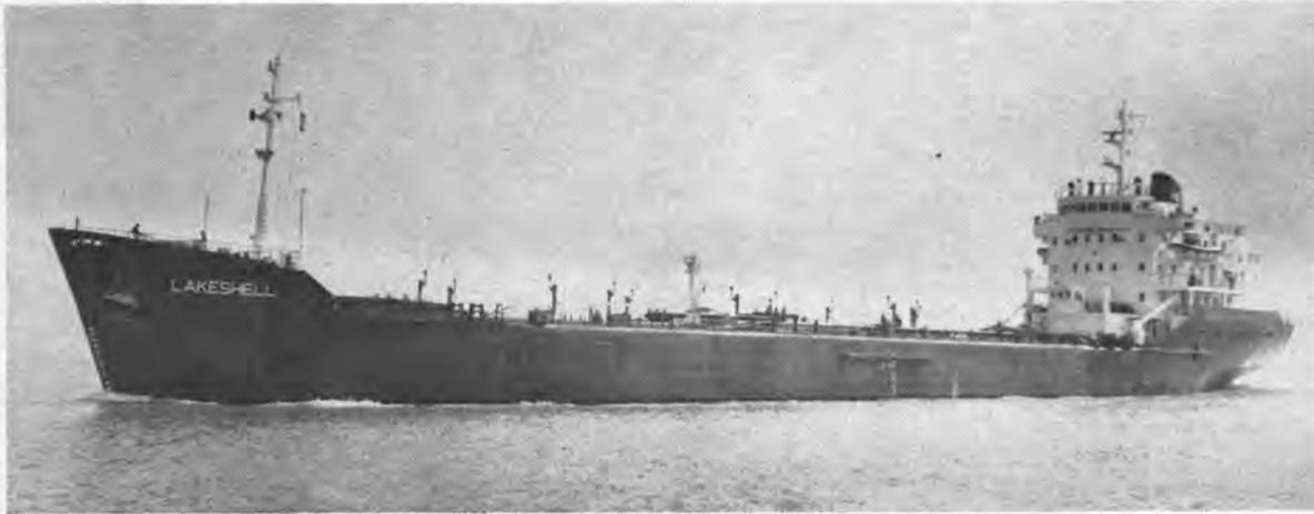
New Shell Canada tanker can handle three separate grades of products simultaneously.
