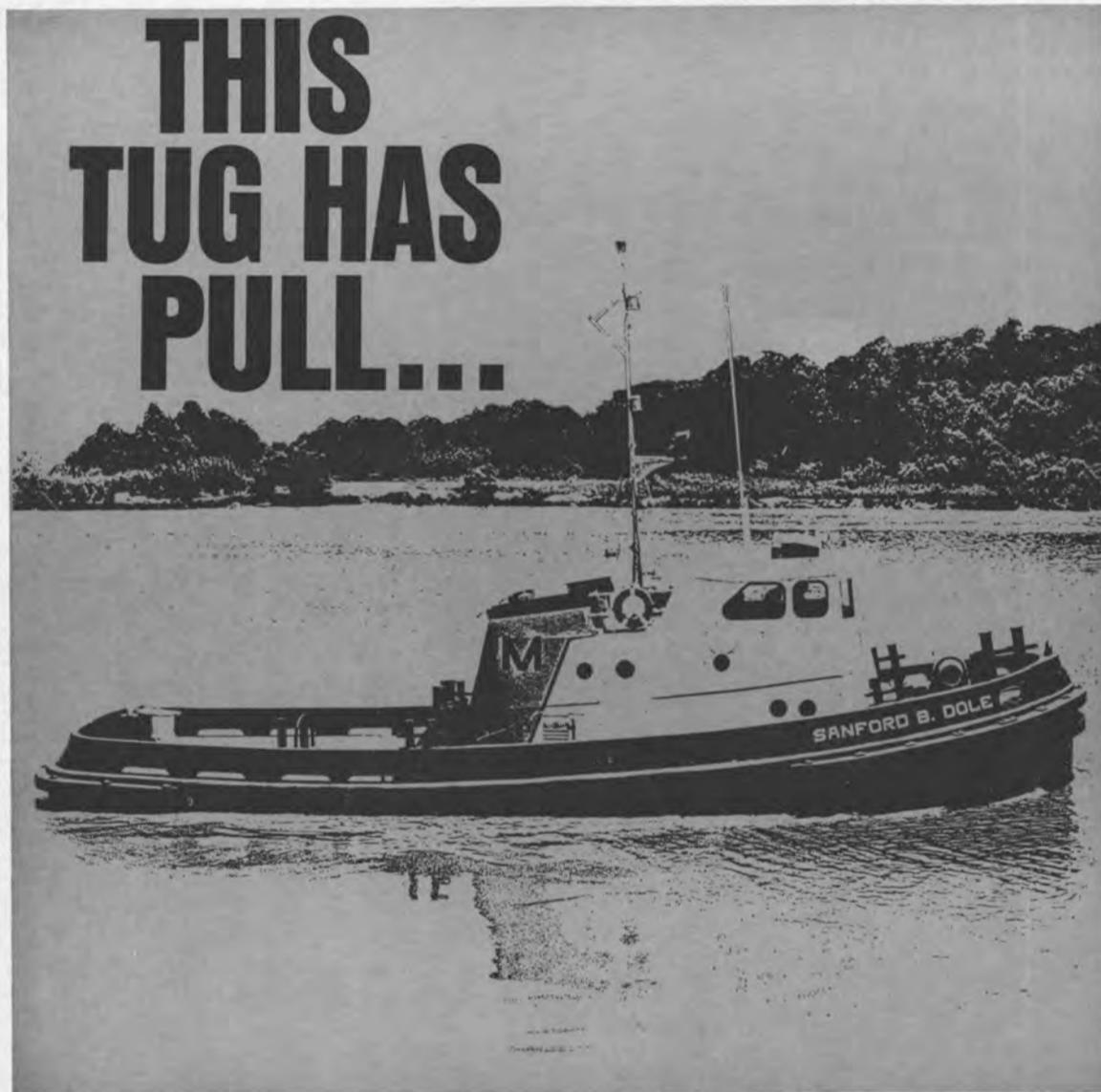
If ever a tug had pull, this one does. Made to take it, powered by two 500 HP Diesel Engines, this tug was delivered to Hawaii to maneuver ocean liners for Matson Navigation. Every piece of her was made to last. 65' x 20' x 10'6" and every inch a champion. Call on the master builders at ZIGLER SHIPYARDS to supply you with a tug that has pull. They never fail.
