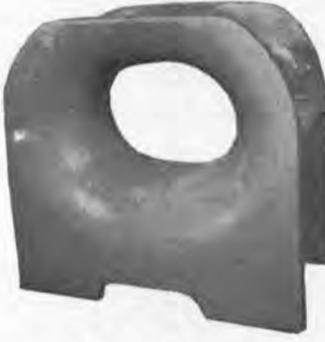
Clear opening 10" x 14" — 7" radius — with extended legs for welding to deck. Use as double or single bow chock. OAL 28" on base — OAW 14" — OAH 27 3/4" — Cast Steel.
