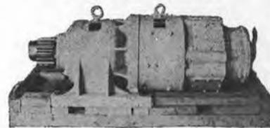
Star Electric Co.—20 HP—230 VDC—73 amps—1200 R.P.M.—compound wound—1 hr. duty—55° rise—with reduction gear 41.2:1—type 5R3165.
