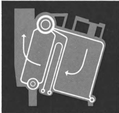
Schematic arrangement of a V2M-8 welded wall marine boiler. Boilers of this type are in fleet use aboard LKA class ships.
