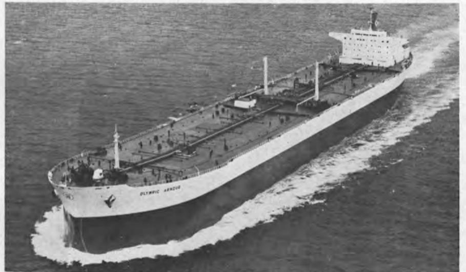
The Olympic Armour, first of five 216,000-dwt sisterships, is designed so that it can pass through the Suez Canal in ballast condition.
