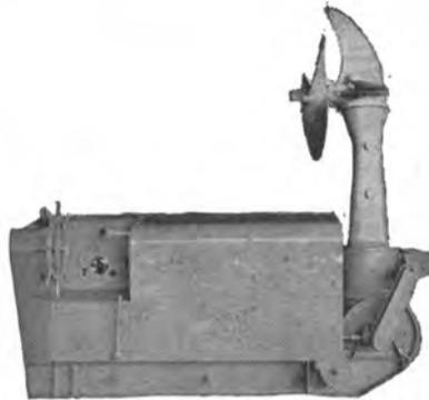
Model 02-D—powered by 6-cylinder G.M. 6-71 diesel—driven through Oliver gear—8708—forward ration 1:1.27—reverse 1:1—3 blade propeller—48" diameter—24" pitch—left hand—manual steering—electric starting. RECONDITIONED—READY TO GO!
