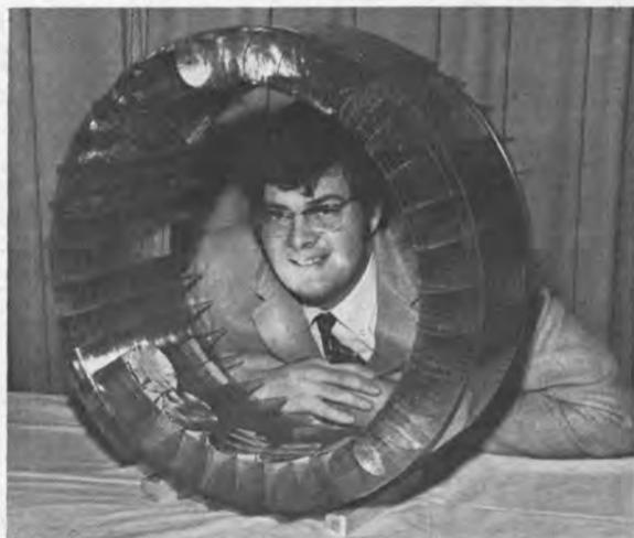
Shaped like a doughnut, this submarine was designed to catch herring efficiently in a net trailed behind the opening. **Paul White**, one of the University of Michigan students on the design team, looks through the opening to show where the trailing net is attached.
