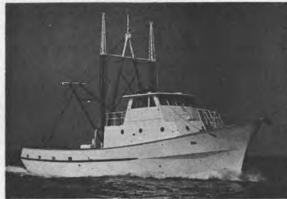
To meet the rising demand for durable and economical shrimp trawlers for long range operation, the Hatteras Yacht Division of North American Rockwell, Inc. has developed a standard 74-foot molded fiberglass trawler. Production has started on this standard trawler in the firm's new New Bern, N.C. facility. The vessel was designed by J. B. Hargrave Naval Architects, Inc., West Palm Beach, Fla.
