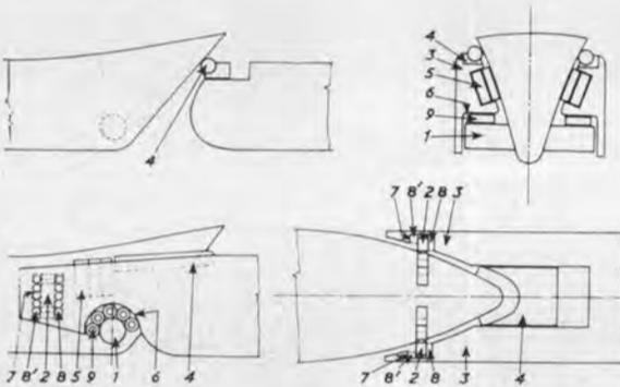
Figure 6—Connection of pusher ship and barge.
