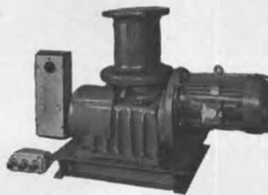
**MOTOR:** 10 HP—totally enclosed—fan cooled—continuous duty—horizontal flange mounted—special shaft & oil seal fitted—440/3/60—1760 RPM. **CONTROL:** Marine type water-tight push-button—forward/reverse/stop—watertight starter box—rated for 40 starts per hour—triple pole contactor with silver contacts, thermal overload relay and trip adjustment. **DIMENSIONS:** Barrel 10" diameter—Flange 10" diameter—approx. 26" wide and 36" long.
