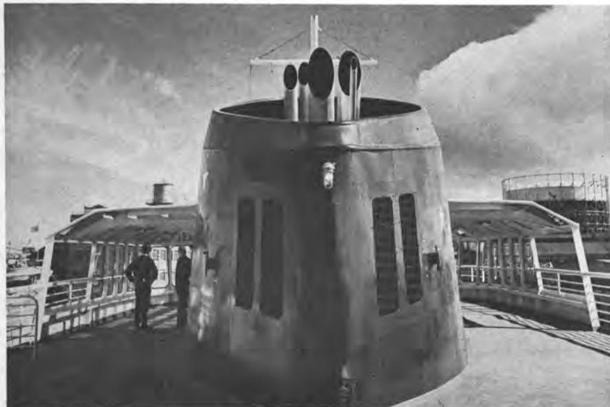
For greater passenger comfort in the new solarium, the height of the stack was increased by three feet. The solarium is heated electrically.
