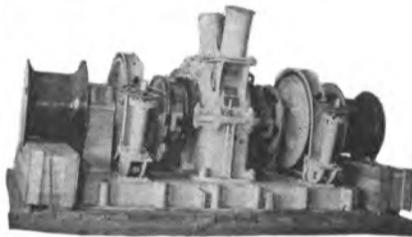
Below deck motor drive. Double Wildcat—driven by 50 HP—230 volt DC motor with vertical shaft and worm drive. Single speed—handles 7000 lb anchors and 60 fathoms of 1 5/8" chain at 7 fathoms per minute. Wildcat centers 56". Complete with all controls and warping features. Total weight 27,500 lbs. With spares.
