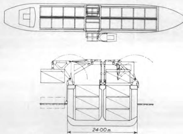
Figure 2—Barge carrier with portal crane.
