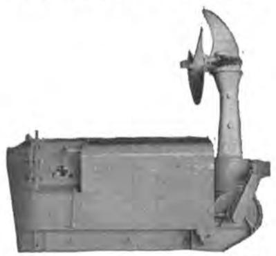
Model 02-D—powered by 6-cylinder G.M. 6-71 diesel—driven through Oliver gear—8708—forward ratio 1:1.27—reverse 1:1—3 blade propeller—48" diameter—24" pitch—left hand—manual steering—electric starting. RECONDITIONED—READY TO GO!
