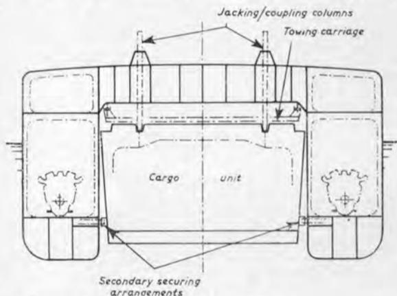
Figure 5—Section through straddler barge carrier.
