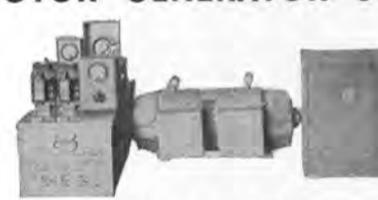
G.E. Type CG-21ACR in a single frame. MOTOR: 5 HP—115 V.D.C.—38 amps—3600 RPM. GENERATOR: 3.5 K.V.A.—2.97 KW—115 volts—1 phase—60 cycle—30.4 amps—model 5LY128A5. DIMENSIONS: 30 3/4" long x 14" wide x 12 3/4" high. Includes magnetic motor starter—Westinghouse 115 V.D.C.—size 3DC—class 6311-531—push button station. Voltage regulator: type CG-23ACE—weight about 800 lbs. each. 2 Boxes of spare parts.
