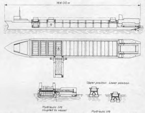
Figure 3—Barge carrier with floodable compartments.
