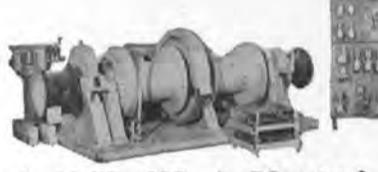
Driven by 10 HP—115 volts DC motor & controls—complete—drums declutchable.
