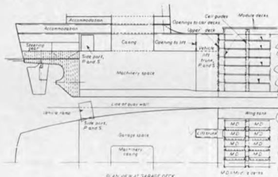
Figure 1—Modular decks in containerships.
