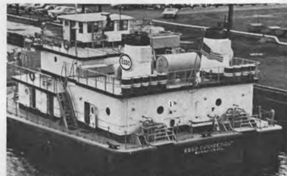
Stern view of new coastal tanker showing the recessed outboard propulsion drive units.
