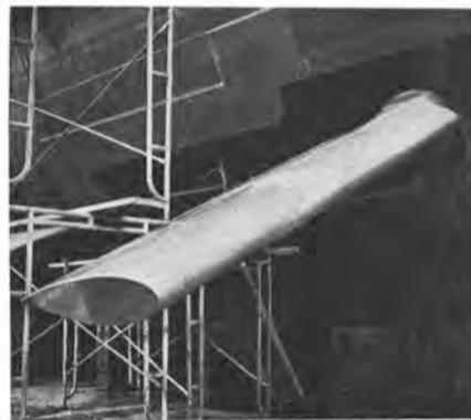
The Tustumena's Pacific Mark X stabilizers are of the horizontal, swing-out oscillating fin type.
