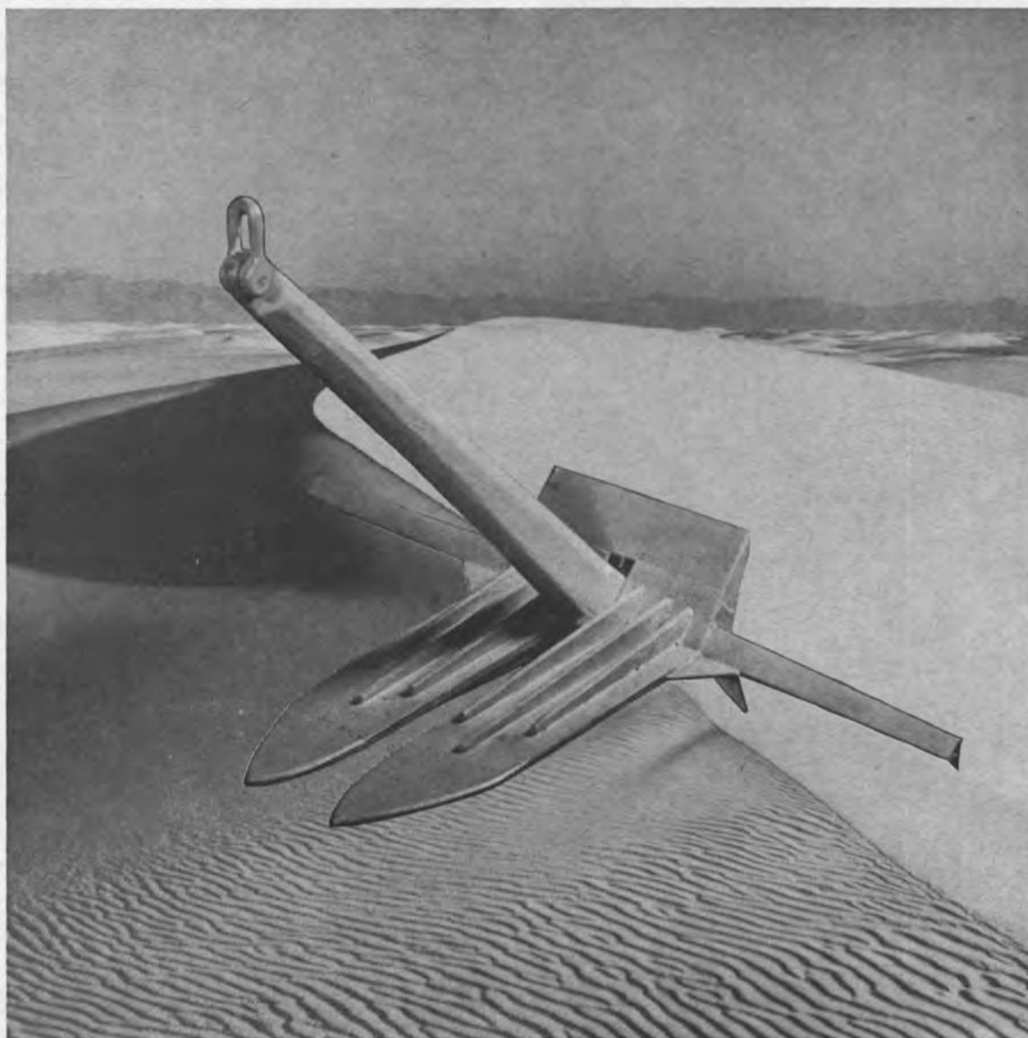
**For Sandy and Soft Bottoms,** specify The Stato®! The Stato is our improved mooring anchor developed for the U. S. Navy affording unusual holding strength in sand and mud. Wedge inserts and palm extensions assure positive fluke tripping and superior holding power.
