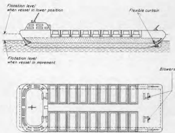
Figure 4—Direct flotation barge carrier.
