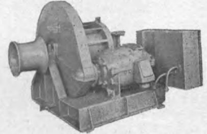
(16) single gear—single drum—7200 lbs. @ 125 FPM. MOTOR: 35 HP—230 VDC—480 RPM—compound—1/2 hour duty. Electric Brake and all controls.
