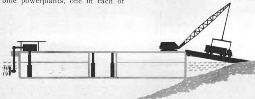
The special barges have their own powerplant, crane and landing bridge all of which stow within the barge when not in use.
