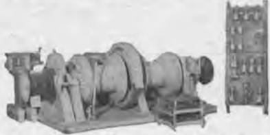
Driven by 10 HP—115 volts DC motor & controls—complete—drums declutchable.
