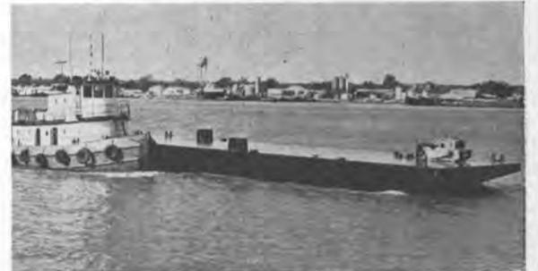
The above photo sequence indicates the unique tilt-table launching system used by Conrad Industries of Morgan City, La. The ARC-23, a 120-foot by 30-foot by 7-foot-3-inch barge built for A. R. Crane Jr., was constructed inside the fabrication building. Upper left photo shows part of the yard force which built the barge with Parker Conrad (far right), president of Conrad Industries, and Frank Elliot (center foreground), barge building superintendent, prior to launching. Upper right
