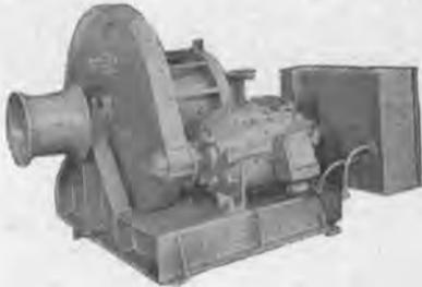
(16) single gear—single drum—7200 lbs. @ 125 FPM. MOTOR: 35 HP—230 VDC—480 RPM—compound—½ hour duty. Electric Brake and all controls.
