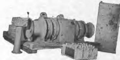
Made by Ideal Electric Co.—with spares. Double wildcat—1-5/16"—15 HP—115 volts DC—1750 RPM—all controls—two outboard gypsies. Wildcats 36" between centers—6000 lb line pull @ 50 FPM. DIMENSIONS: O.A. width over gypsies—84"; OA length 81". Will sell windlass without power if desired.
