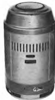
The all-in-one design, ideal for wheelhouse installation, also provides the ultimate in safety. It is compact, impervious to variations of ambient temperature and has punctiform suspension in lieu of the conventional gimbal system to insure a low natural frequency of the compass system and a steady compass read-out.
