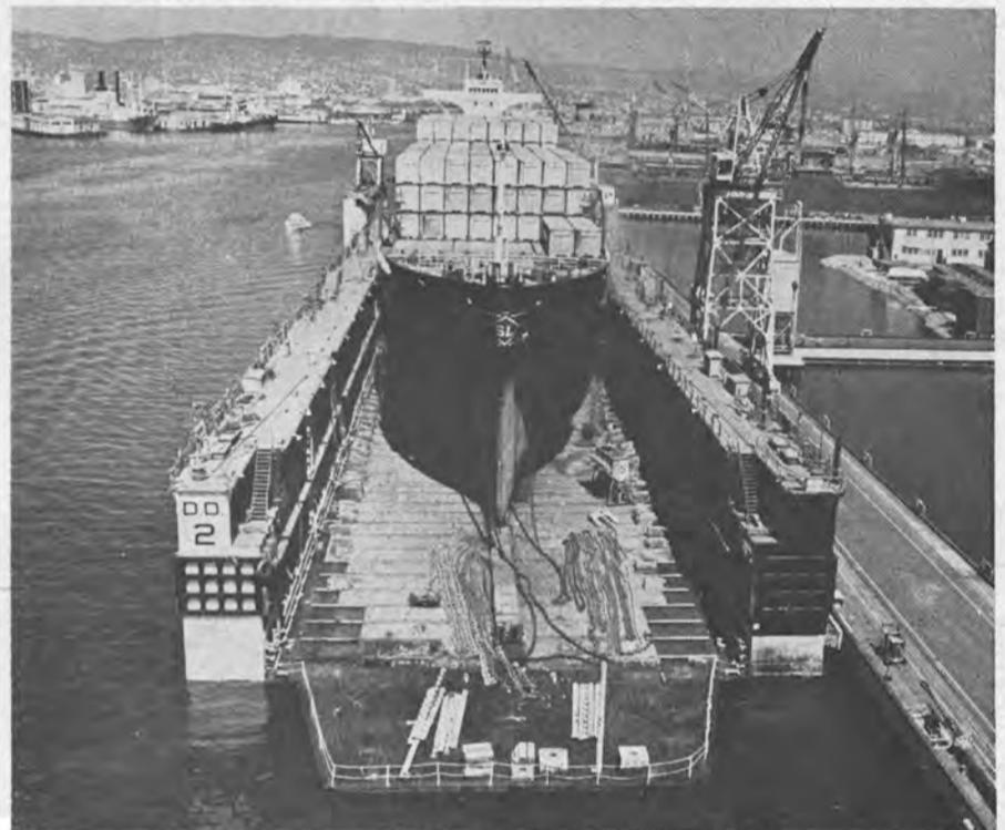
Sea-Land's containership Oakland is the first vessel to test Todd-Alameda yard's new heavy-lift floating dry dock. The new dock has a capacity of 25,000 tons.
