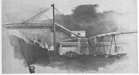
Unique 33-ton container crane to be installed at the Port of Los Angeles will ride with rear legs on top of existing warehouse building. In addition to containers, a grab bucket attachment will enable the crane to unload bulk products. Curve in tracks in artist's rendering allows gantry structure to negotiate a turn on the wharf.
