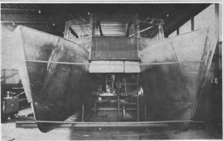
**CATAMARAN SURVEY VESSEL** under construction at Fercraft Marine Inc., La Prairie, Quebec, Canada for the Canadian Department of Transport. The 50-foot vessel was designed by **Robert B. Harris**, naval architect, Great Neck, N.Y., for survey work in the Gulf of St. Lawrence. With 600-hp diesel propulsion, the boat will have a cruising speed of 17.4 knots and a maximum speed of 21.5 knots.
