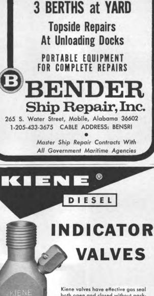
both open and closed without pack-ing or glands. Operates against pressure — will never blow open. Small and rugged — 4¼" in length with only 3¼" circle of space for attachments. Kiene valves give better service under the most severe conditions. Standard indicator plug and wing nut connection.
