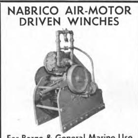
For Barge & General Marine Use Winch duty 11,000 lbs. @ 39 FPM. Drum capacwinch duty 11,000 lbs. @ 39 FPM. Drum capac-ity 115 ft. of 1" wire. Drum size-11". Air motor mfg by Gardner-Denver-type MKB-A-reversible -11.5 HP @ 100 lbs. pressure. 1" Pipe con-nections for air. Typical serial No. 458307. Just removed from unmanned barge. Good operating condition. 7 Units, with motors, available.
