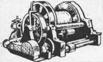
Single drum, capacity 2000' of 2" wire rope, cylinder size 9" bore by 10" stroke.
