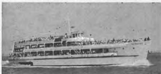
1100 passengers, 92 gross tons, three decks, 2 lounges, 165' x 36' x 5'5" draft loaded, speed 14 knots with two 6-71 Quads total 1320 hp. Generators (2) 3-71 20kw 120 volt DC, Decca 303 radar, Fathometer, Sperry steerer. Vessel built 1944, with major widening and conversion 1959 and 1966.
