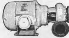
1—GOULDS, 2000 GPM, 470' head, size 8 x 10, Westinghouse Motor, 350 HP, 2300/3/60.
