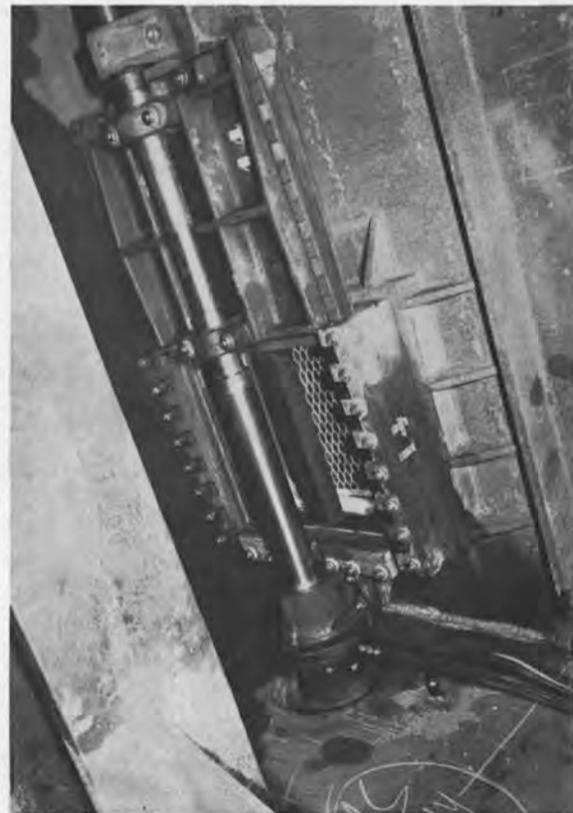
SIGMA type port valve in bulkhead provides for the inter-tank free-flow system and greatly reduces cargo piping.
