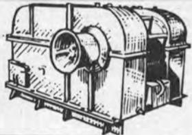
LAKESHORE UNIWINCHES, with Allis-Chalmers Motors, 50 HP, 230 Volts DC, complete with Control Equipment.
