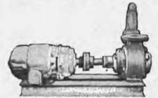
6—WORTHINGTON, Size 8L1, 2100 GPM, 138.5 TDM, with Westinghouse motor, 100 HP, 230 DC.
