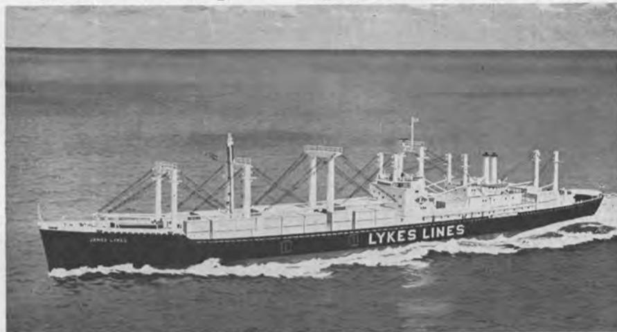
This is how the newly lengthened ships of the fleet of Lykes Bros. Steamship Co., Inc., look after adding a new 97-foot mid-body section. Todd Shipyards in Galveston are converting the ships at a cost of \$30 million.
