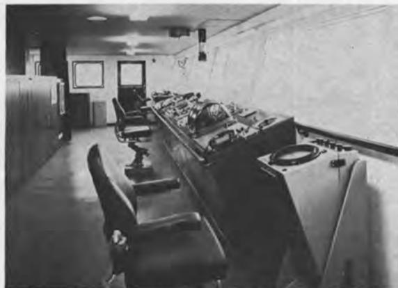
The large wheelhouse has navigating, steering and machinery controls in one console along forward bulkhead.
