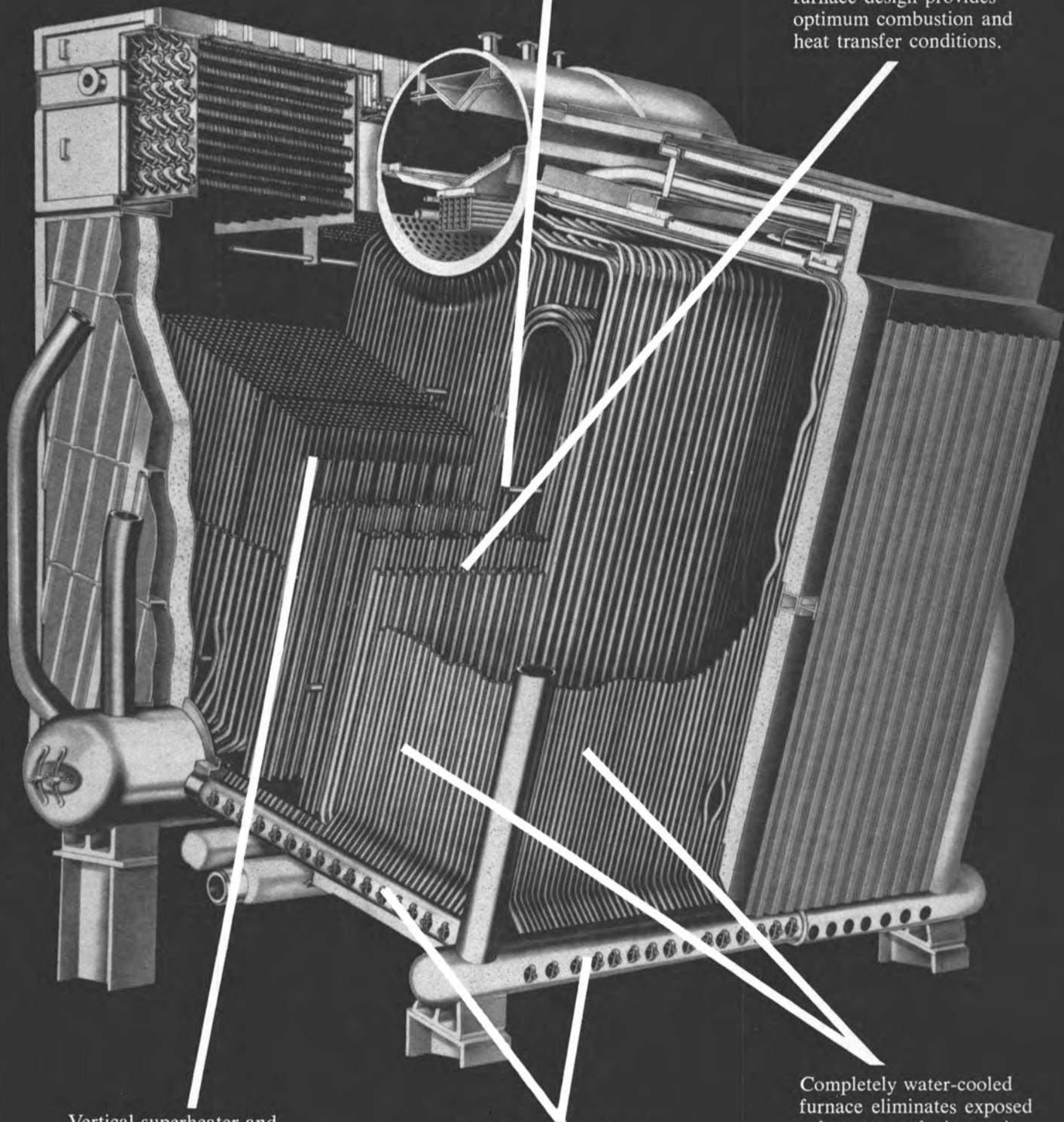
Vertical superheater and in-line boiler tubes minimize slugging and improve efficiency.
