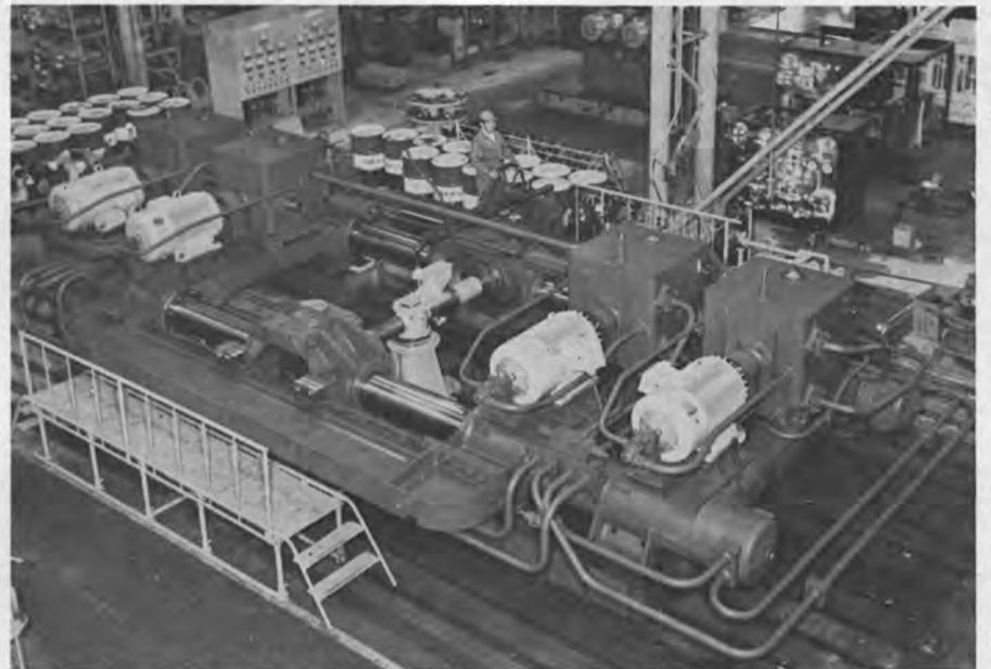
World's largest electro-hydraulic steering gear assembled in Kawasaki Heavy Industries' shop for testing. The overall width of the unit is 33 feet 11 inches and it measures 17 feet 4 inches in the fore-and-aft direction. Its height is 6 feet 5 inches.
