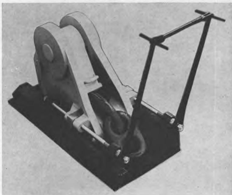
One unit can eliminate devil's claws, turnbuckles, bow stoppers and, it utilizes less space. The one stopper that serves the dual purpose of transferring chain load to the vessel's structure and houses the chain in a snugly stowed position.
