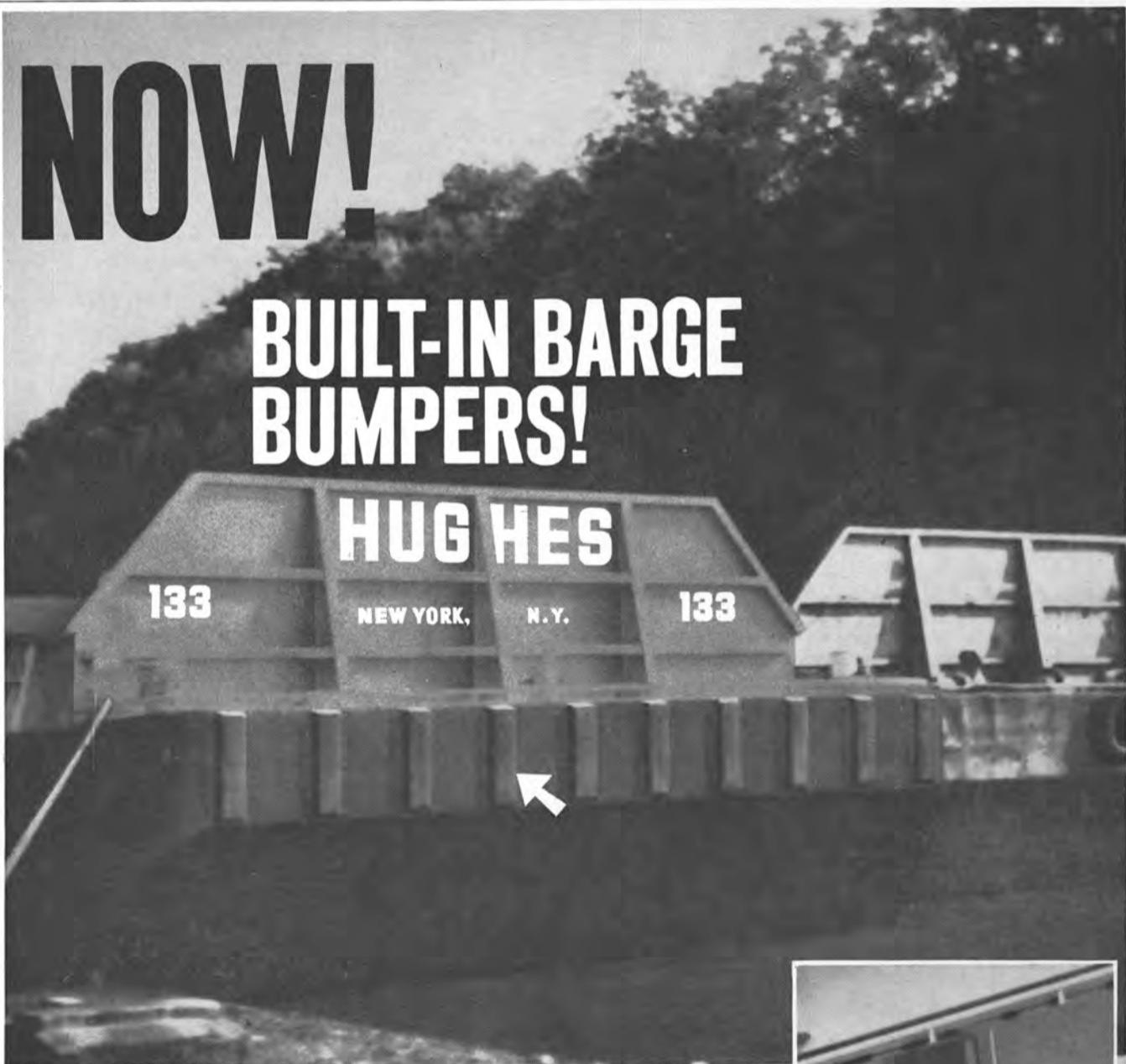
**PROTECTO-HULL, developed by HUGHES, produced by UNIROYAL, prevents costly lay-ups and repairs!** Once installed, PROTECTO-HULL fenders are on to stay. Bonded to a steel plate the units are welded to the hull. They won't fall off, can't be sheared off. Performance-tested more than two years, they've proven their worth and their permanence. Easy to install on existing craft or during construction. For details, phone or write:
