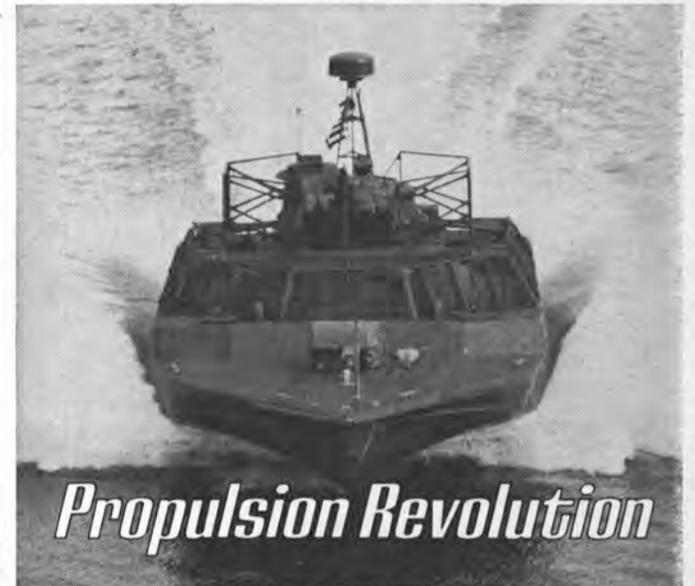
Assault Support Patrol Boat—Three 20-inch Turbopower units.
