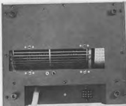
View of programmable control unit, showing some of the 40 punched metalized cards pre-programmed for particular frequencies. Cards can be changed in minutes, even at sea.
