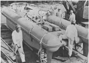
The catamaran-type hulls on the vehicle are fabricated of ASTM A36 steel plate of 26-inch diameter.
