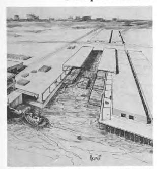
This architect's rendering shows the Port of Galveston's barge-carrying ship berth and covered barge terminal for loading/unloading and interchange, located on Galveston's Piers 34 and 35. Construction is under way on this facility and it will be ready to receive barges and ships later this year.
