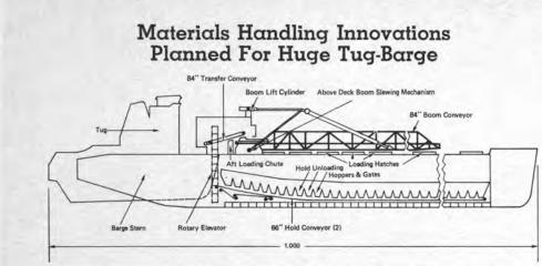
Schematic drawing of tug-barge cargo transporter shows layout of materials handling system which includes a total of 198 unloading hoppers, dual 66-inch-wide hold conveyors, unique rotary elevator, transfer conveyor and 250-foot boom conveyor.
