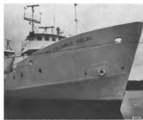
The \$1.4-million R/V Columbus Iselin, shown at dockside in the Bellinger Shipyards, Jacksonville, Fla. Fortyfoot-long steel plates, supplied by Republic Steel's Gadsden, Ala., mill, were used for its construction and in the making of the molded hull.
