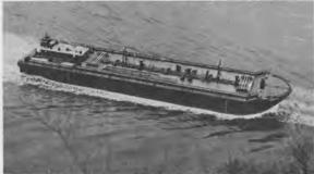
The Seaspan 822, shown above, is designed to be towed either off the nose or using West Coast bridles and is rigged for either mode of towing.
