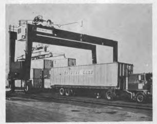
Paceco 40-long-ton Transtainer at the Port of Norfolk, Va., similar to the two Transtainers to be installed at the North Point Wharves.
